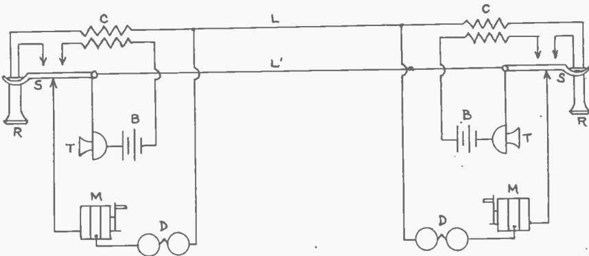
FIG. 1. CONNECTION OF "SERIES" TELEPHONES.
