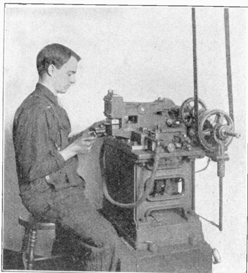
WELDING BUCKLES WITH THE AUTOMATIC ELECTRIC WELDER.
