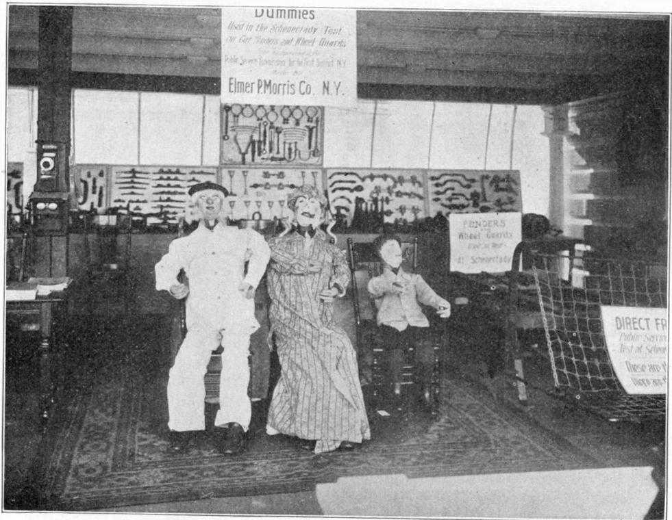
FIG. 1. STREET CAR FENDER AND DUMMIES USED IN TESTING.
