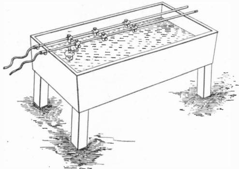
FIG. 1. ELECTROPLATING ON GLASS.
