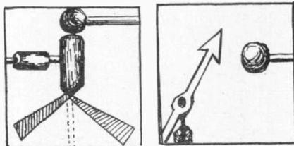
FIG. 5. FOIL ELECTROSCOPE. FIG. 6. ARROW ELECTROSCOPE.
