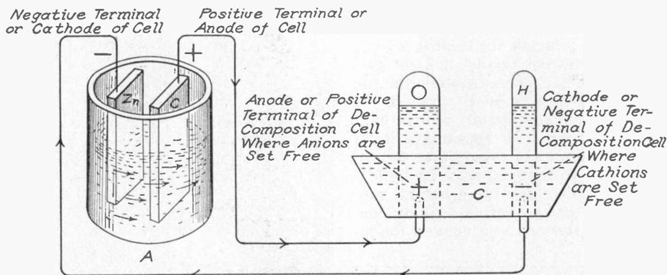
FIG. 70. ELECTROLYTIC DECOMPOSITION OF WATER.
