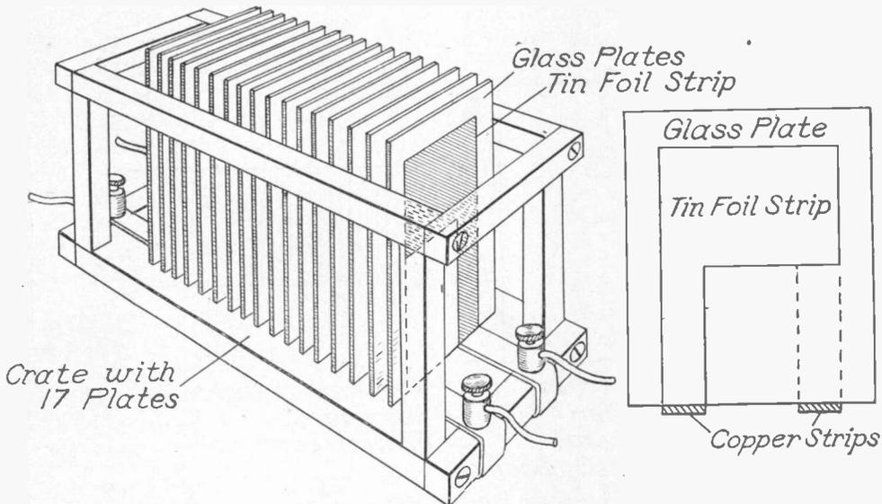
FIG. 2. CONDENSER FOR HIGH FREQUENCY APPARATUS.
