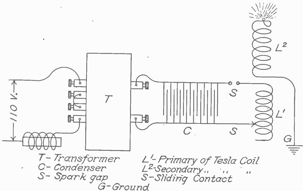
FIG. 3. CONNECTIONS FOR HIGH FREQUENCY APPARATUS.
