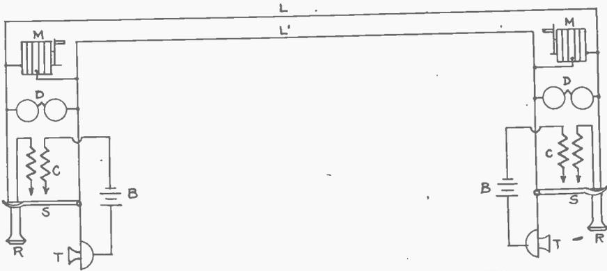
FIG. 2. CONNECTION OF "BRIDGING" TELEPHONES.
