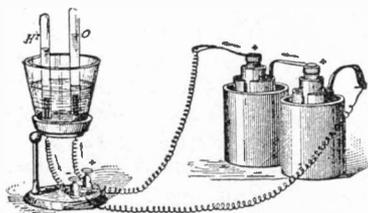
FIG. 69. APPARATUS FOR THE ELECTROLYSIS OF WATER.
