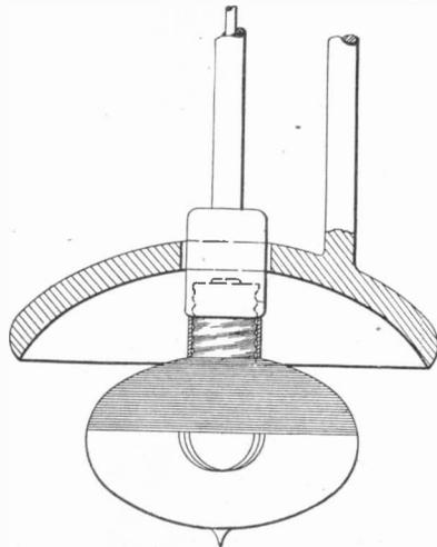
FIG. 2. ARRANGEMENT FOR ELECTROPLATING LAMP BULB.
