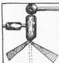
FIG. 5. FOIL ELEC-TROSCOPE.
