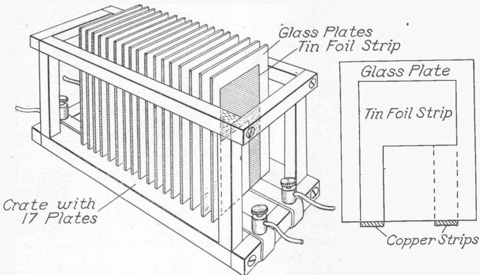
FIG. 2. CONDENSER FOR HIGH FREQUENCY APPARATUS.
