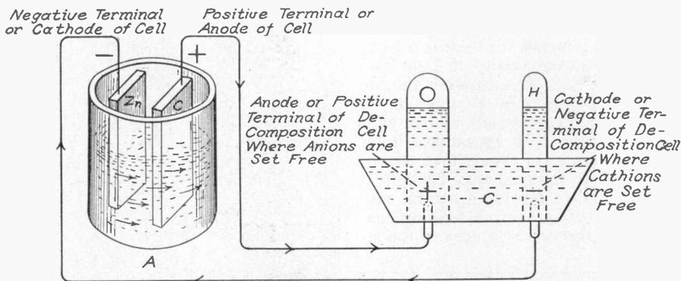
FIG. 70. ELECTROLYTIC DECOMPOSITION OF WATER.
