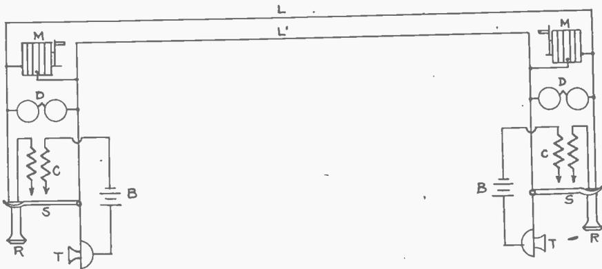
FIG. 2. CONNECTION OF "BRIDGING" TELEPHONES.
