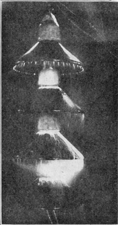
TESTING A HIGH TENSION INSULATOR.
