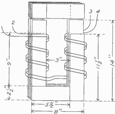
Connect No. 2 and 4 together for series connection and for parallel No. 1 & 2, And also 3 and 4.
