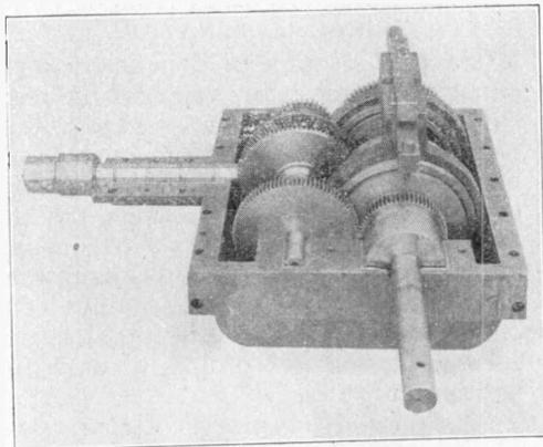
CLUTCH MECHANISM FOR MOTOR DRIVEN PLANER.
