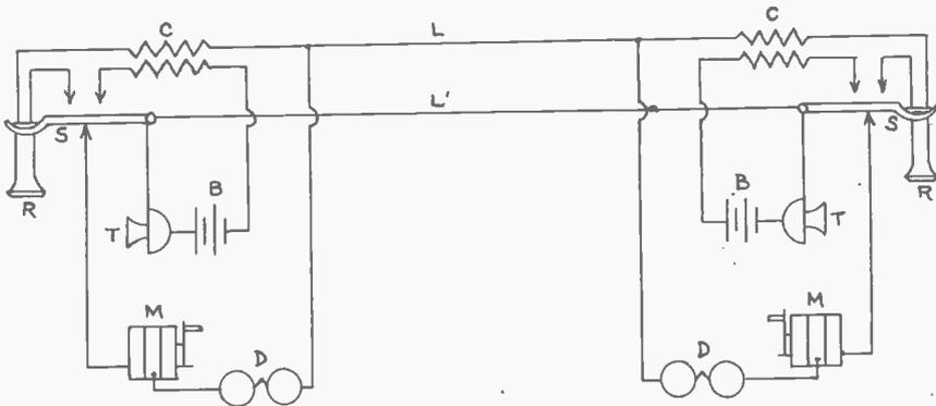
FIG. 1. CONNECTION OF "SERIES" TELEPHONES.
