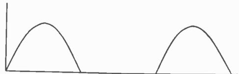
FIG. 13. CURRENT WOULD FLOW ONLY HALF THE TIME
