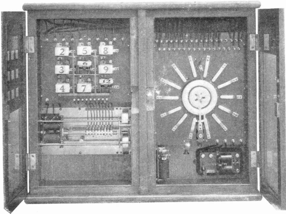
TESTING APPARATUS FOR AUTOMATIC JOURNAL ALARM
