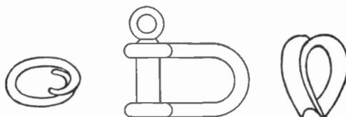
FIG. 9. WIRE ROPE THIMBLES AND SHACKEL BOLT
