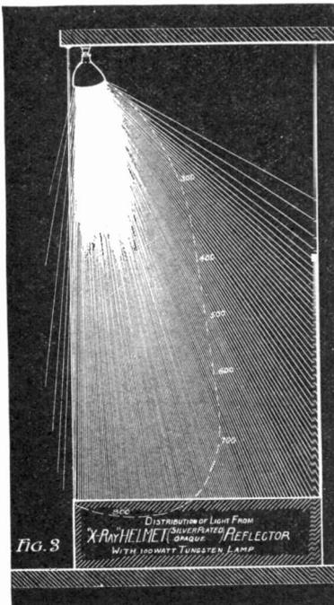
The principle of efficient show window lighting demands that lamps be placed high up in the front of the window and out of sight of the passer-by. Also, the light must be strong in the window and minimum out on the sidewalk. The cuts illustrate the difference between efficient and inefficient lighting, being drawn on the plan employed by illuminating experts to illustrate intensity of light distribution.
