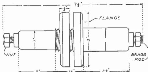
FIG. 13. DETAILS OF BUSHING
