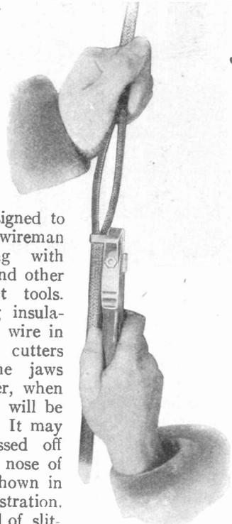
The method of slitting the insulation on SLITTING INSULATION duplex wire is shown in the third illustration and is very simple, being done with the cutting jaws. These jaws are forced through the insulation and the pliers drawn toward the operator, the insulation being cut as rapidly and as clean as a piece of cloth with a sharp pair of scissors.
