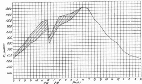
FIGS. 164 AND 165. LOAD CURVES OF LIGHTING STATIONS, SHADED PORTIONS SHOWING LOAD DUE TO ELECTRIC IRONS
