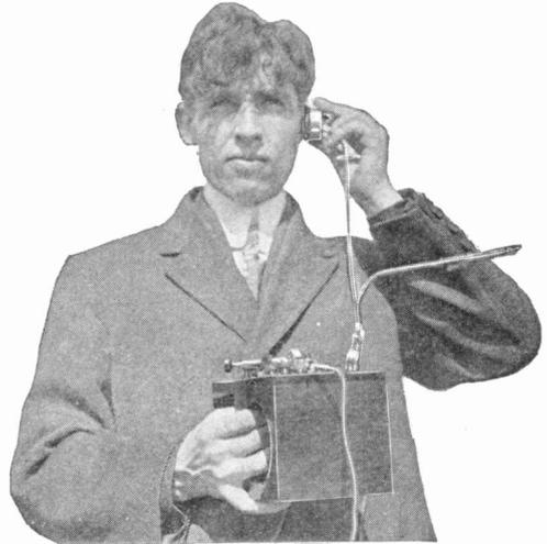
RECEIVING A WIRELESS MESSAGE FROM AN AEROPLANE IN FLIGHT
