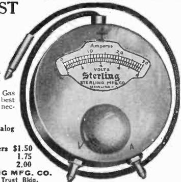
These instruments are designed for all kinds of Automobiles, Motor Boats, Gas Engines, Etc. The best wherever testing is necessary.
