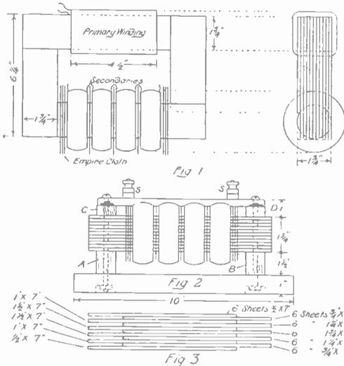
DETAILS OF CLOSED CORE TRANSFORMER.
