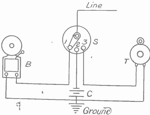
CONNECTIONS FOR SIMPLE TELEPHONE SYSTEM
