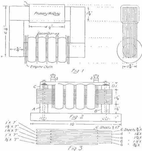
DETAILS OF CLOSED CORE TRANSFORMER.
