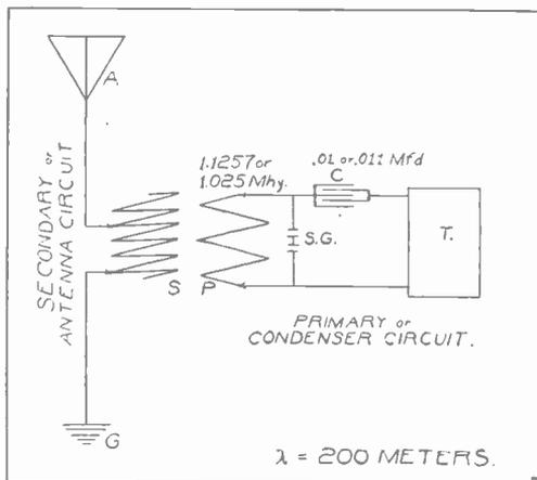
FIG. 4. A—AERIAL; G—GROUND; L—INDUCTANCE WITH PRIMARY P AND SECONDARY S; S.G.—SPARK GAP; C—CAPACITY; T—TRANSFORMER
