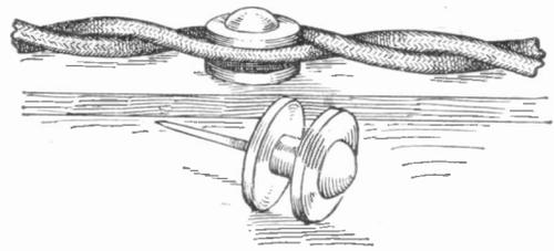
This trouble may be eliminated by using the Eureka insulated nail, the collar of which, as shown, prevents any undue pressure upon the insulation of the wire and further provides additional insulation between the wires and the metal of the nail.
