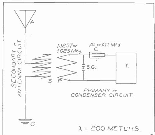
FIG. 4. A—AERIAL; G—GROUND; L—INDUCTANCE WITH PRIMARY P AND SECONDARY S; S.G.—SPARK GAP; C—CAPACITY; T—TRANSFORMER
