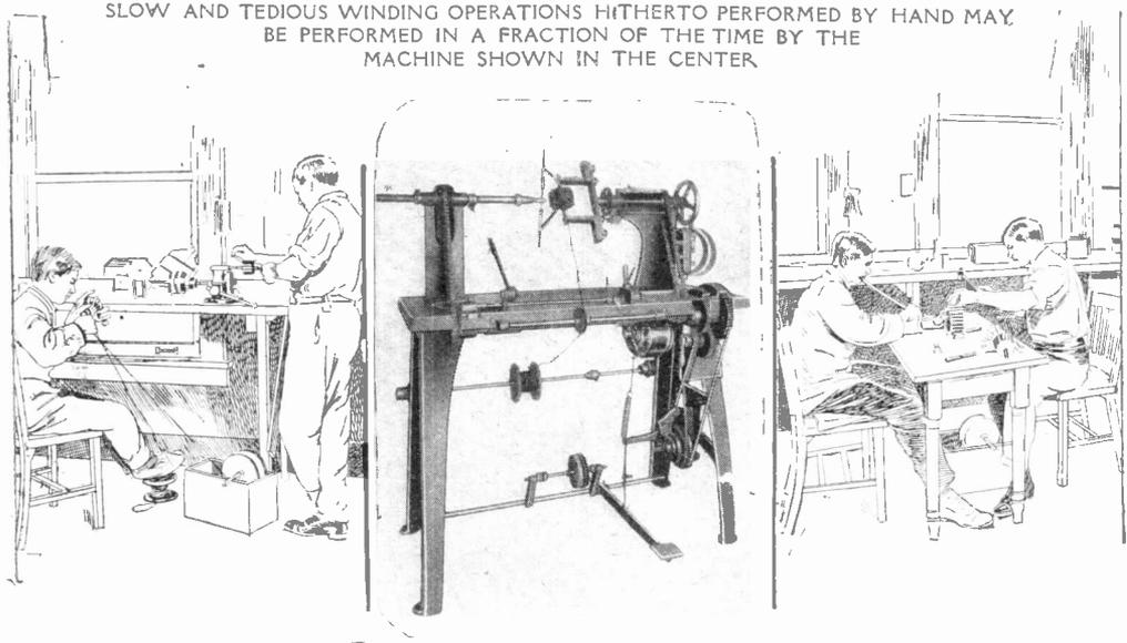
winding a drum armature and a ring armature. Yet so flexible is the machine that in a few moments it may be adjusted to do either. In addition it winds solenoid coils, transformer fields and induction coils; even more, it embodies an adjustable coil form, a very simple device which, attached to the winder, actually forms up the coils, after they are wound, to any desired shape.
