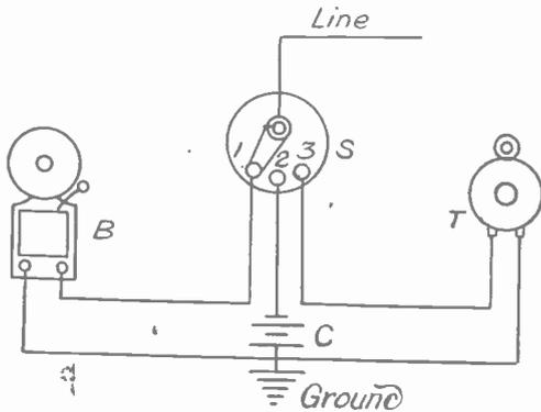
CONNECTIONS FOR SIMPLE TELEPHONE SYSTEM
