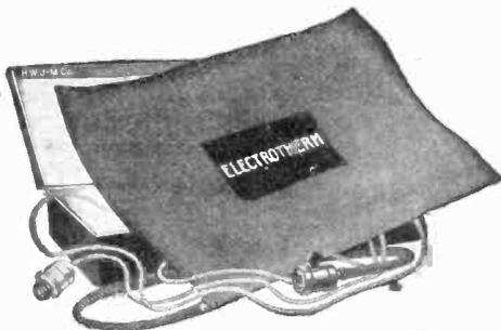
It consists of a thin, light and flexible sheet or pad containing wires insulated and protected with Asbestos. When attached to an ordinary incandescent lamp socket, it offers sufficient resistance to the current to produce a constant and uniform degree of heat. It is provided with a regulating switch by means of which three different temperatures can be obtained.
