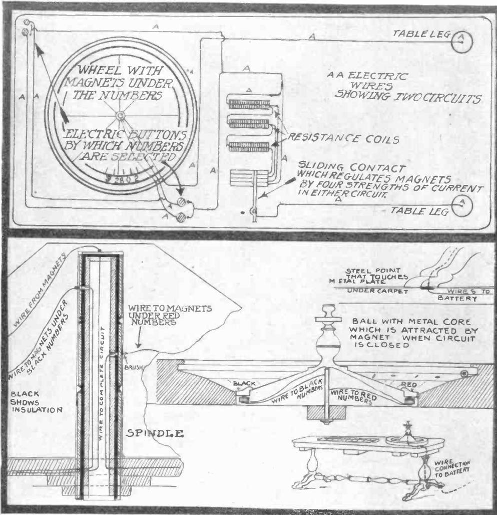
LAYOUT AND CONNECTIONS OF THE CROOKED ROULETTE WHEEL
