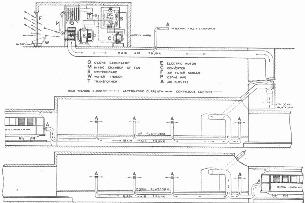
DIAGRAM SHOWING THE "OZONAIR" SYSTEM IN THE TUBES OF THE CENTRAL LONDON RAILWAY
