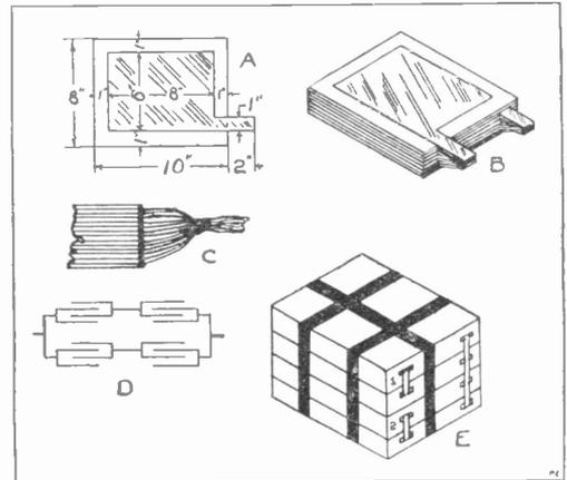
FIG. 5. A—DIMENSIONS OF FOIL AND GLASS PLATE; B—ASSEMBLED PARTS; C—DETAIL OF LUG; D—SERIES-PARALLEL CONNECTIONS; E—FOUR UNITS IN SERIES-PARALLEL
