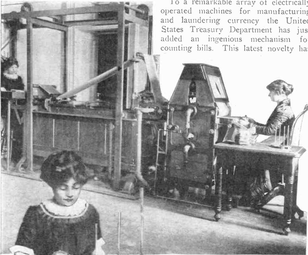
To a remarkable array of electrically operated machines for manufacturing and laundering currency the United States Treasury Department has just added an ingenious mechanism for counting bills. This latest novelty has
