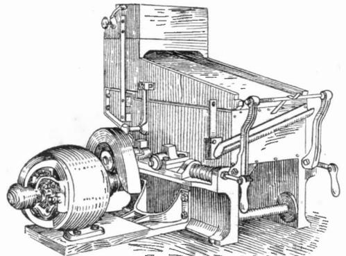
MACHINE FOR CRUSHING OATS
