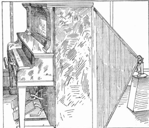
METHOD OF DIRECTING THE SOUND WAVES INTO THE TRANSMITTER
