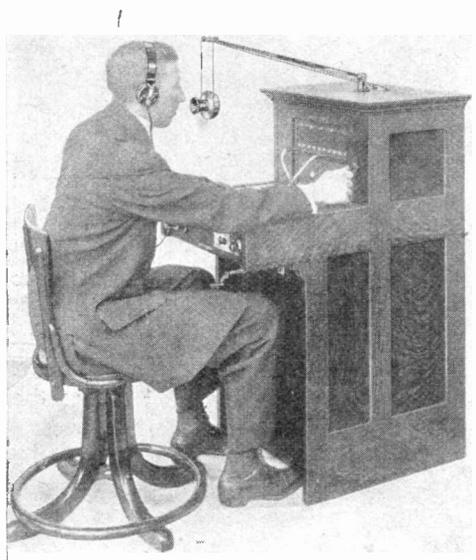
COMMON TYPE OF PRIVATE EXCHANGE SWITCHBOARD EASILY FITTED WITH THE NEW CODE CALL KEY
