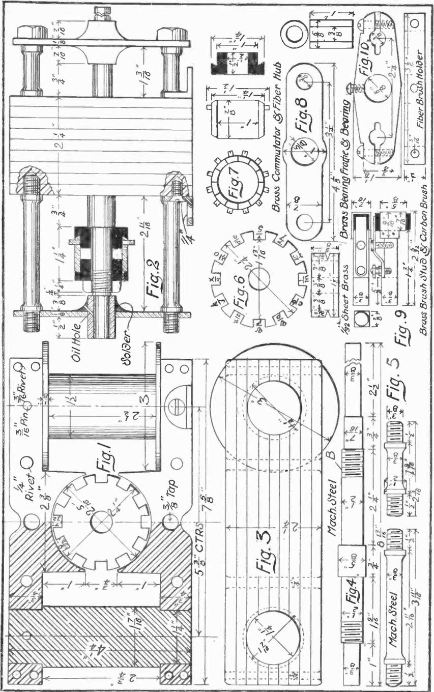
To insulate the armature cover the shaft next to the armature with  $1/32$  inch sheet fiber  $3/4$  inch wide. Make two  $1/16$  inch fiber washers  $2\frac{1}{4}$  inches in diameter, slip them on the ends of the shaft and glue them to the ends of the armature. After the glue has set cut out the slots. Make twelve channel pieces out of  $1/32$  inch sheet fiber and glue them into the slots and to the fiber washers; when set trim off with a sharp knife and be sure to have all the iron covered.
