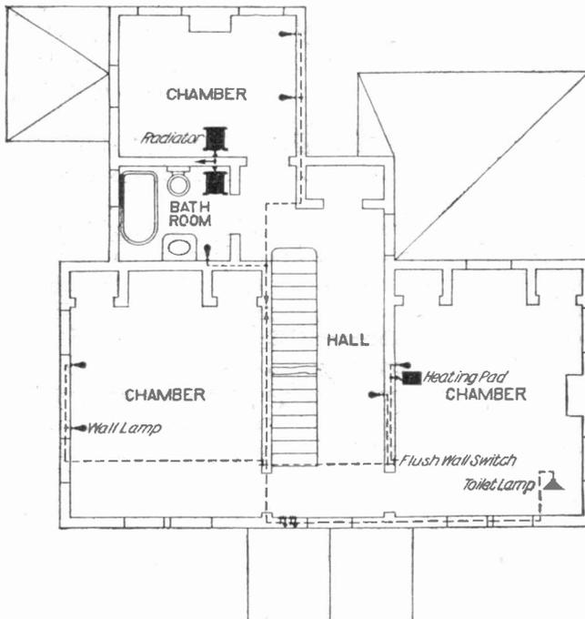
PLANS FOR A HOUSE COSTING LESS THAN \$5,000, IN WHICH THE WIRING CIRCUITS HAVE BEEN PROPERLY ARRANGED TO GIVE OUTLETS AND SWITCHES IN THE RIGHT LOCATIONS
