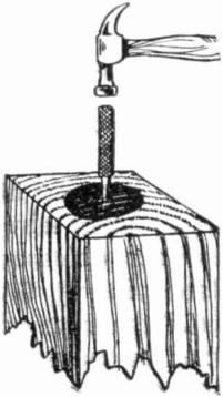
To make holes in armature laminations or other pieces of sheet metal, place the metal upon a block of wood, the grain of which is cut so as to pound directly at the end of the grain. Use a flat ended punch, and strike a sharp, quick blow with a fairly heavy iron. In this way a clean-cuthole will be made, while if a sharp-pointed punch is employed, the metal will be pushed aside instead of being punched, and leave a ragged edge inside the hole.
