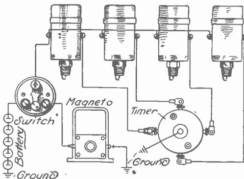
CONNECTIONS OF COMBINATION SPARK PLUG AND COIL
