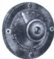
Below is the Dubilier Variadon as supplied from the factory with graduated scale and knob
