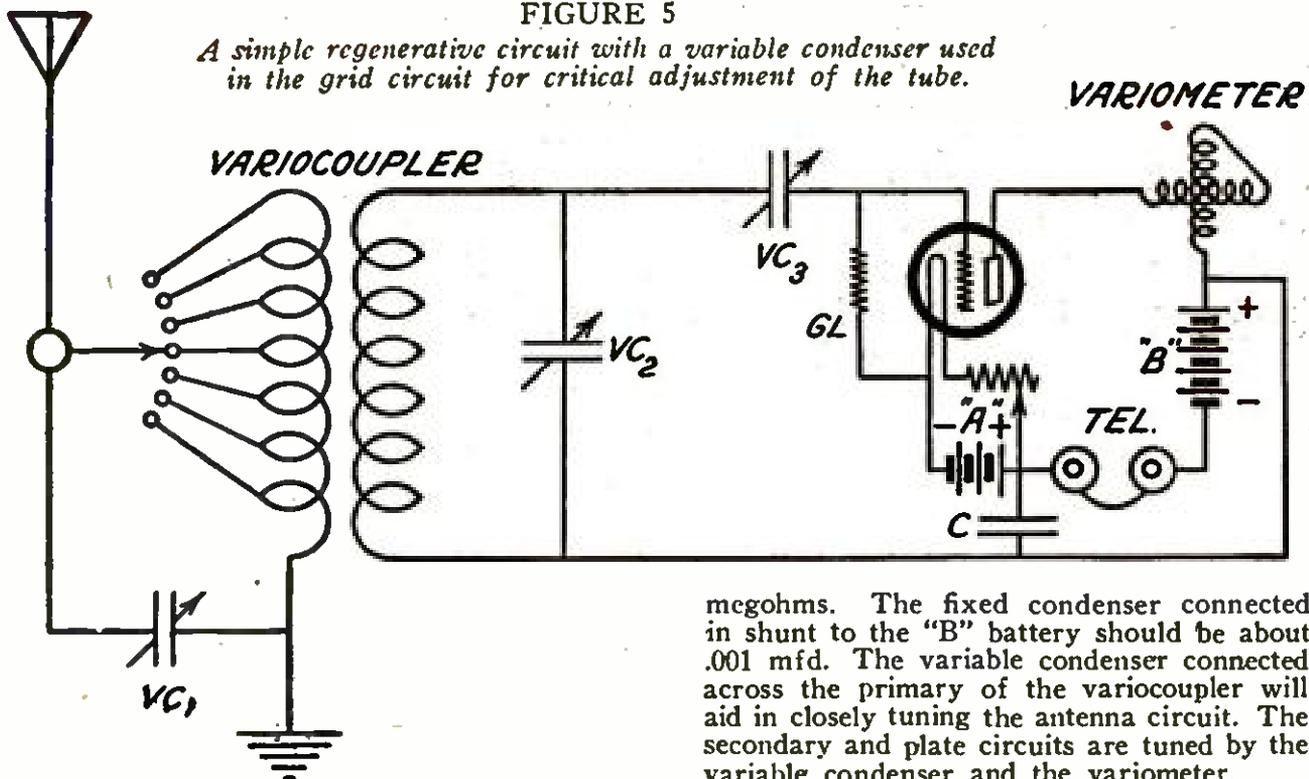
megohms. The fixed condenser connected in shunt to the "B" battery should be about .001 mfd. The variable condenser connected across the primary of the variocoupler will aid in closely tuning the antenna circuit. The secondary and plate circuits are tuned by the variable condenser and the variometer.
