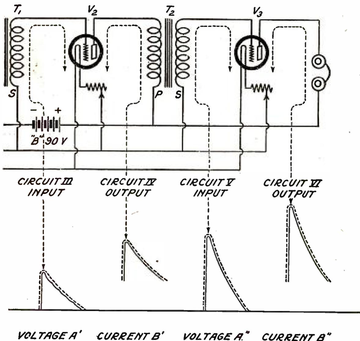
winding P by means of the bypass condenser C, and only the audio frequency component of the current B (which is shown by the dotted lines) passes through the winding P. This current, flowing through P, induces a similar impulse in the secondary winding S, except that the voltage of the impulse induced across the Circuit 3 is higher than the voltage in Circuit 2 on account of the step-up ratio used in the transformer windings.
