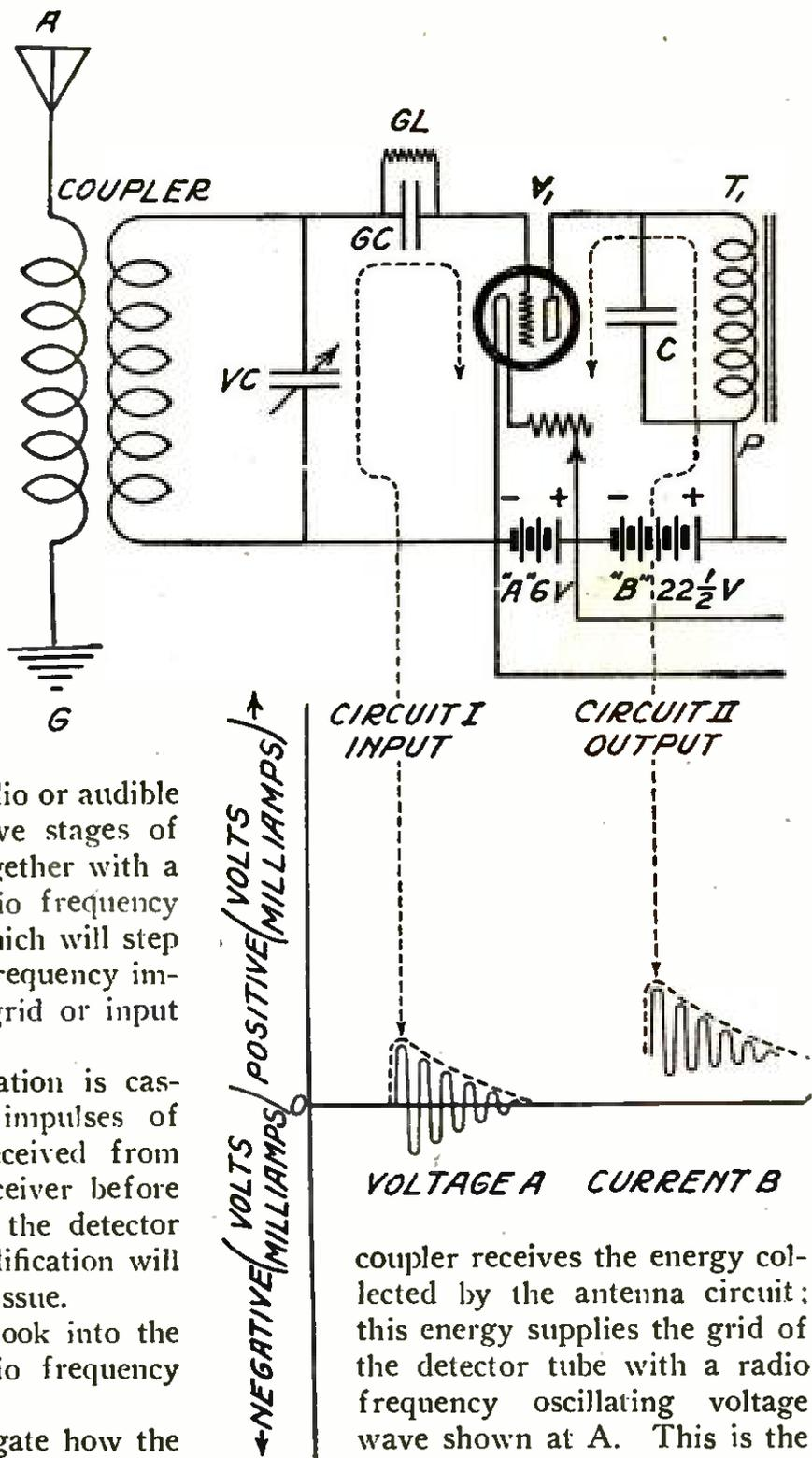
coupler receives the energy collected by the antenna circuit; this energy supplies the grid of the detector tube with a radio frequency oscillating voltage wave shown at A. This is the voltage across the circuit designated as Circuit 1.
