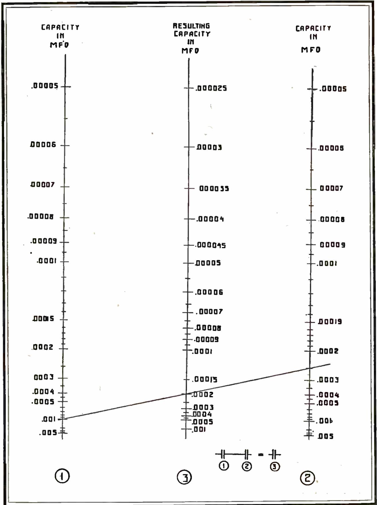
**A CHART FOR CALCULATING THE CAPACITY OF CONDENSERS IN SERIES**
