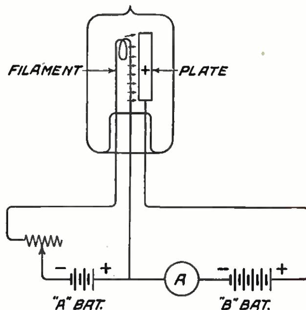
**HOW THE FLEMING VALVE WORKS**
