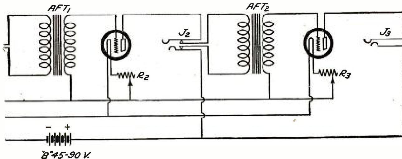
UV-200 tube for the detector, with 22½ volts on the plate.
