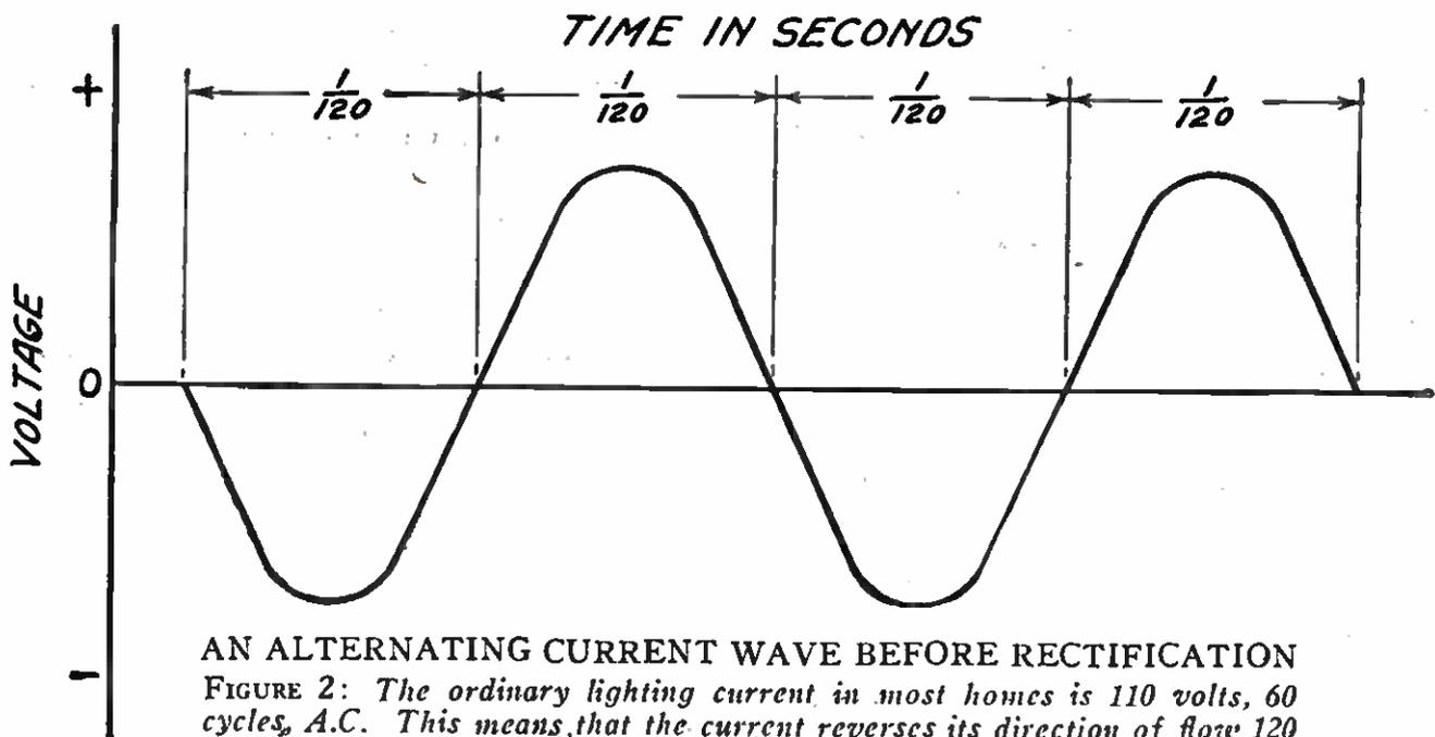
AN ALTERNATING CURRENT WAVE BEFORE RECTIFICATION
