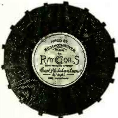
RayCoils "A" for Reinartz, Ray Coils "B" for RCS and Ultra Audion Circuits, RayCoils "C" for RCS, Ultra Audion and Tuned Radio Frequency for All Circuits. RayCoils "D" for Neutralizing Circuits 4 & 5 Tubes.
