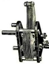
The Kellogg Switchboard & Supply Company have just placed on the market a standard Il plate variable condenser of minimum .000074 and maximum. 00035 microfarads, and has as part of its construction a micrometer vernier condenser with a capacity minimum of one micro-microfarad and a maxi-
