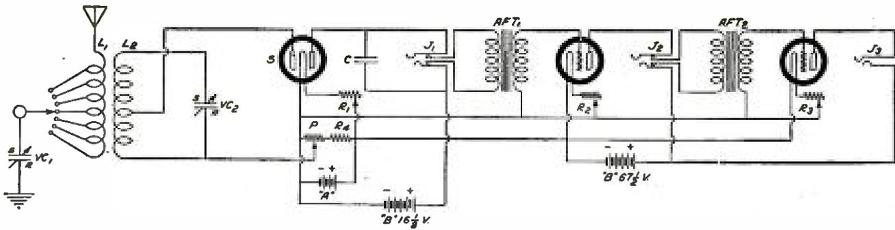
**DONLE DETECTOR CIRCUIT WITH TWO STAGES OF AUDIO-FREQUENCY AMPLIFICATION**
