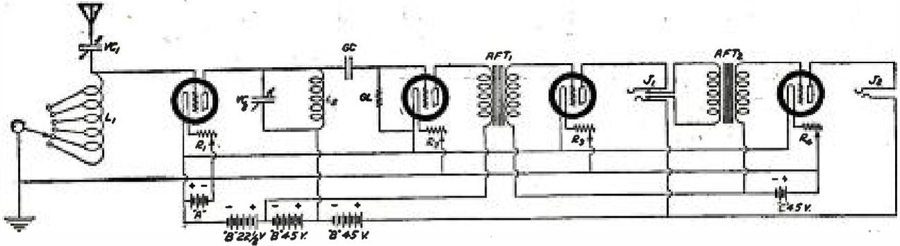
ONE STAGE OF TUNED-RADIO-FREQUENCY, DETECTOR AND TWO STAGES OF AUDIO-FREQUENCY AMPLIFICATION
