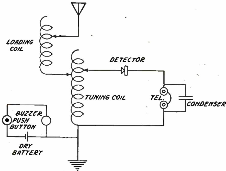
**CONDUCTIVELY-COUPLED CRYSTAL SET WITH LOADING COIL AND BUZZER TEST**
