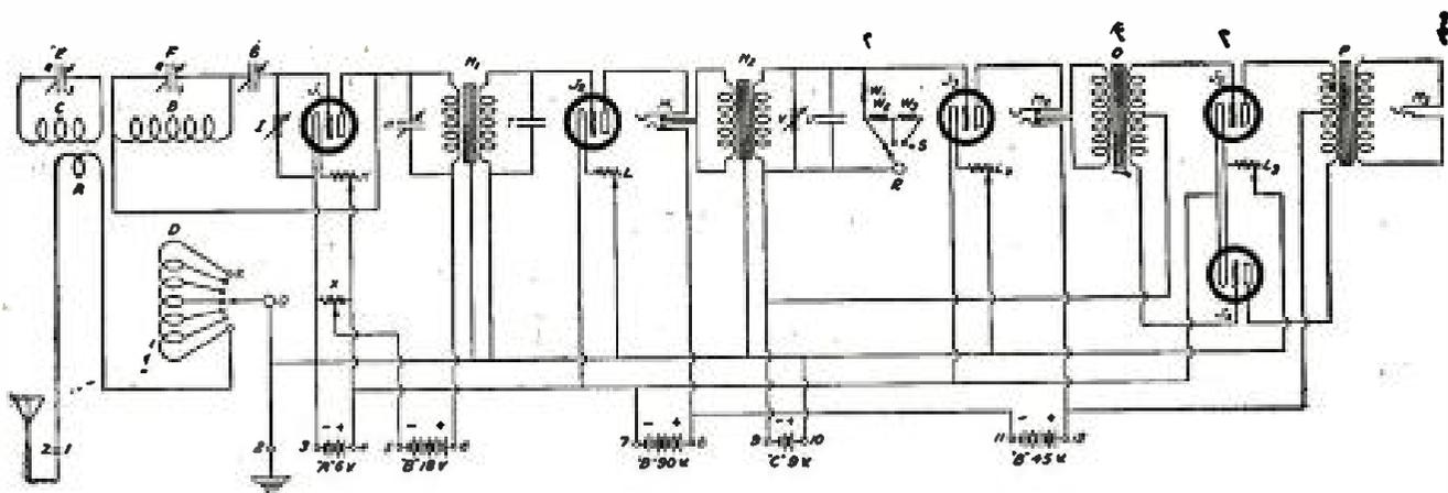
THE FOUR-CIRCUIT TUNER WITH TWO STAGES OF STRAIGHT TRANSFORMER-COUPLED AMPLIFICATION, AND ONE STAGE OF PUSH-PULL AMPLIFICATION
