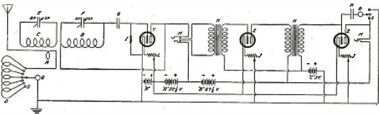
THE THREE-TUBE, 4-CIRCUIT TUNER
