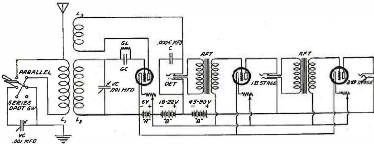
TRIPLE-COIL, HONEYCOMB REGENERATIVE CIRCUIT WITH TWO STAGES OF AMPLIFICATION
