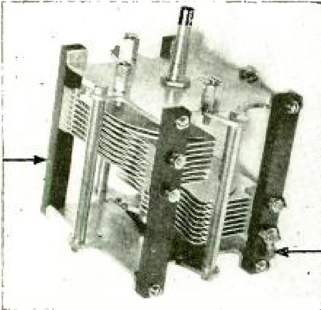
*Radion separators are used on this condenser with soldering lugs for connections.*
