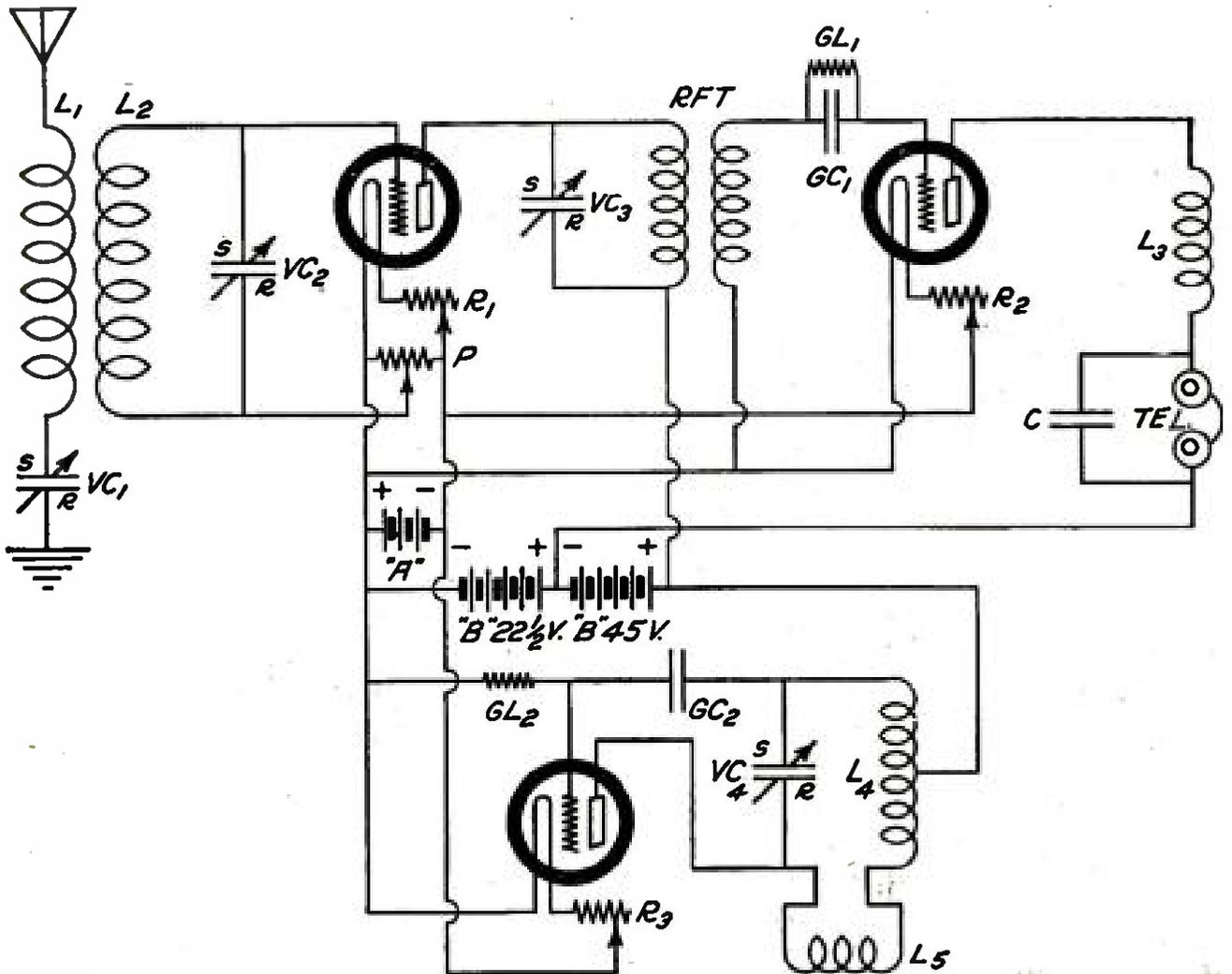
ONE STAGE OF TUNED-RADIO-FREQUENCY, VACUUM-TUBE DETECTOR, WITH SEPARATE HETERODYNE FOR CW RECEPTION
