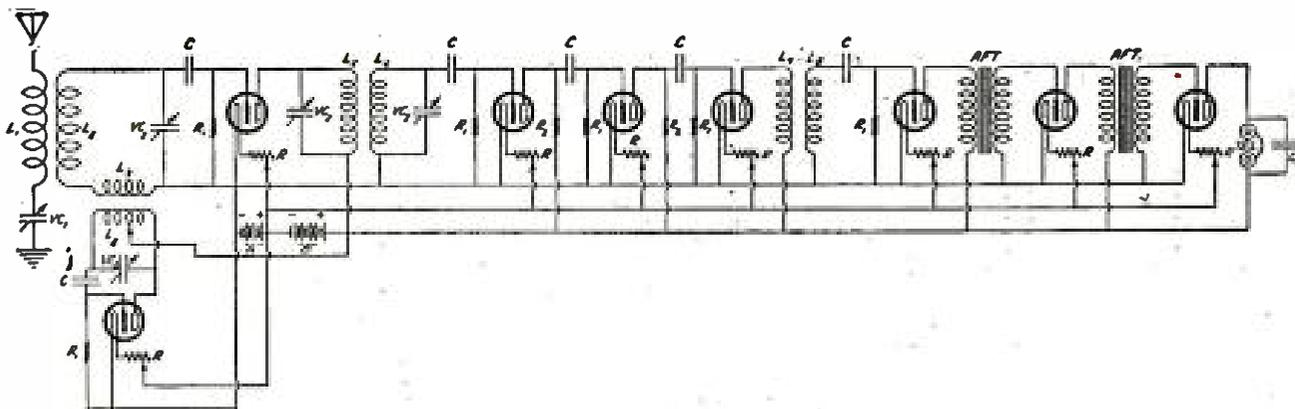
A RESISTANCE-COUPLED SUPERHETERODYNE WITH TWO STAGES OF AUDIO-FREQUENCY AMPLIFICATION
