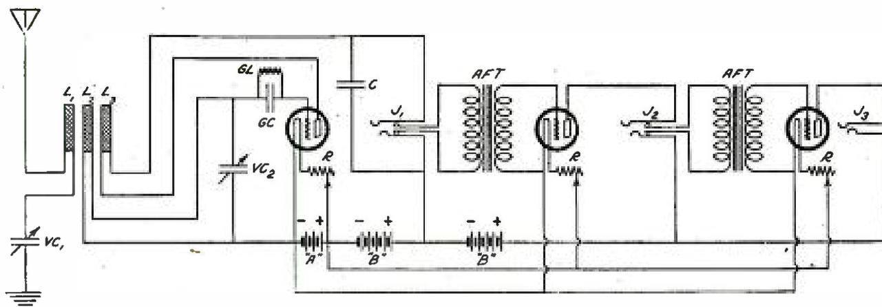
TRIPLE-COIL HONEYCOMB REGENERATIVE RECEIVER WITH TWO STAGES OF AUDIO-FREQUENCY AMPLIFICATION
