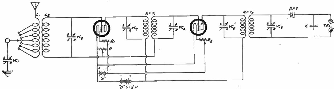
CIRCUIT EMPLOYING TWO STAGES OF TUNED-RADIO-FREQUENCY AMPLIFICATION, WITH A CRYSTAL DETECTOR
