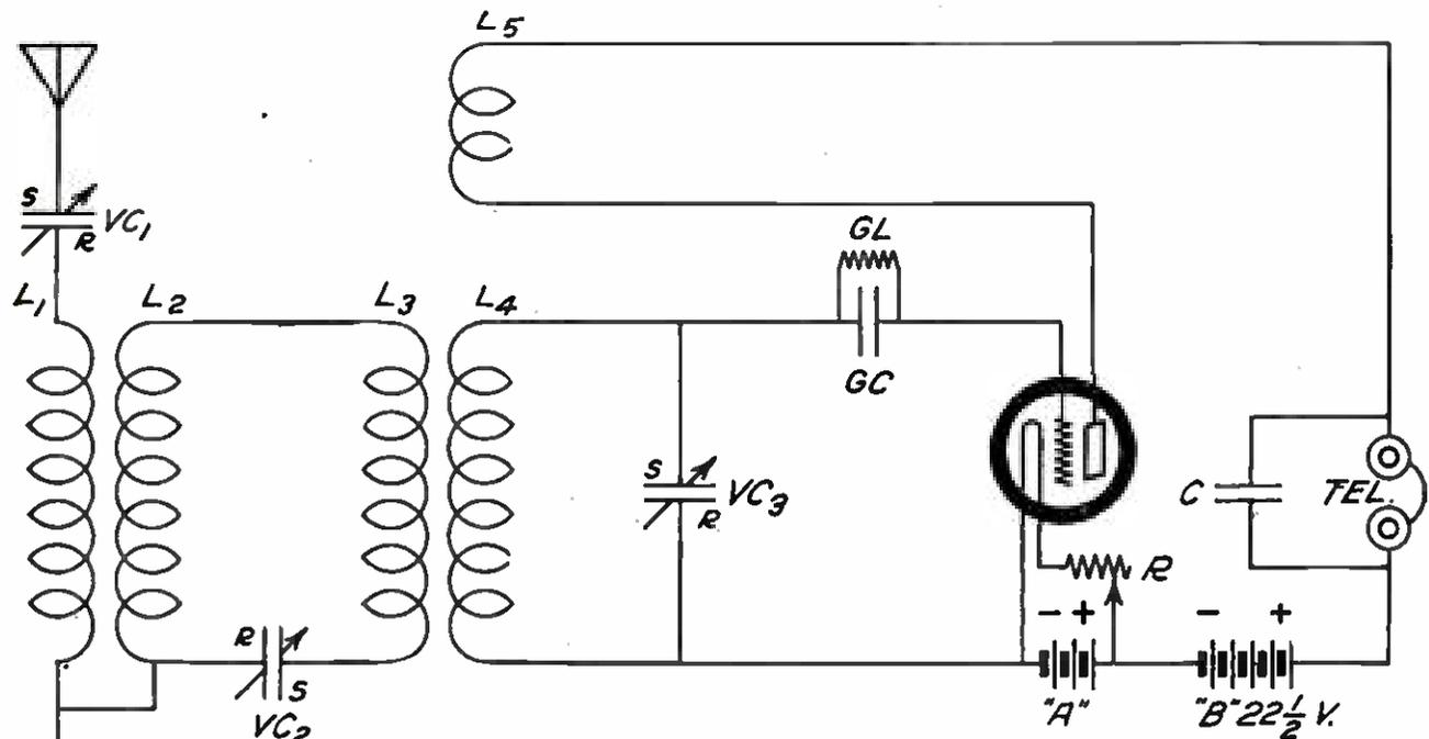
A REGENERATIVE RECEIVER WITH AN INTERMEDIATE CIRCUIT TO REDUCE RADIATION
