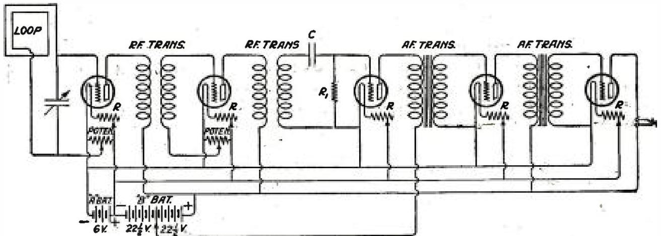
TWO STAGES OF RADIO, DETECTOR, AND TWO STAGES OF AUDIO-FREQUENCY AMPLIFICATION
