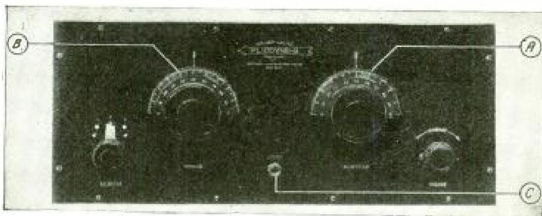
*A and B are the tuning dials. C is the loudspeaker jack.*
