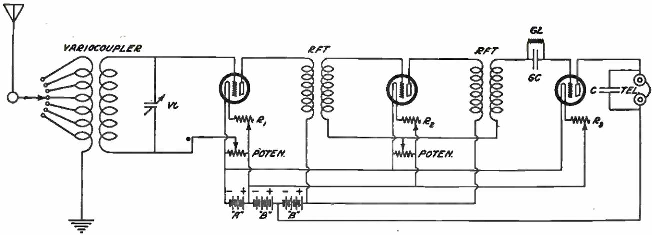
TRANSFORMER-COUPLED RADIO-FREQUENCY CIRCUIT WITH VACUUM-TUBE DETECTOR
