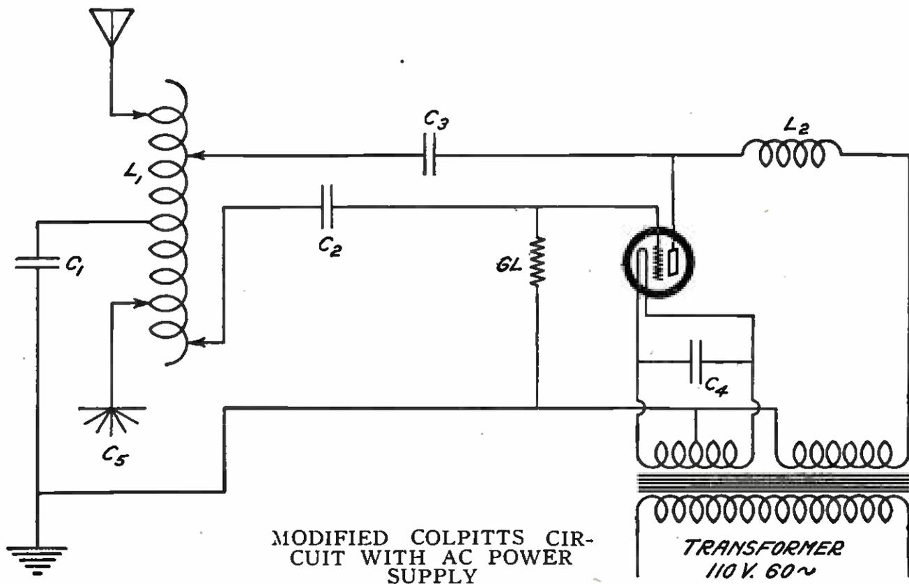
MODIFIED COLPITTS CIRCUIT WITH AC POWER SUPPLY
