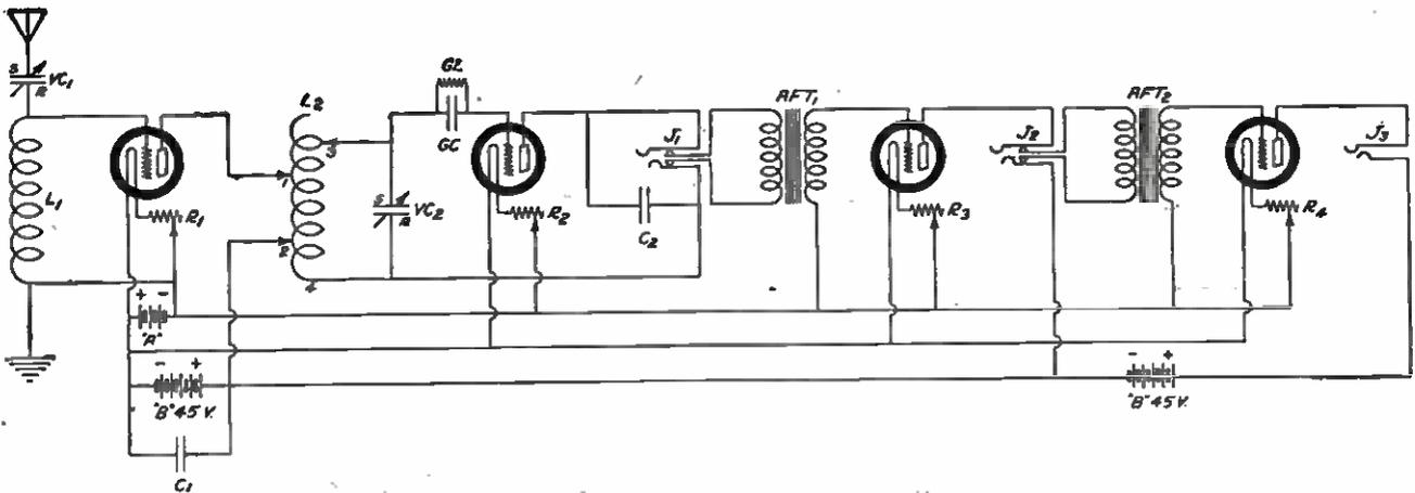
ABELE CIRCUIT COMPRISING ONE STAGE OF TUNED-RADIO-FREQUENCY AMPLIFICATION, VACUUM-TUBE DETECTOR AND TWO STAGES OF AUDIO-FREQUENCY AMPLIFICATION
