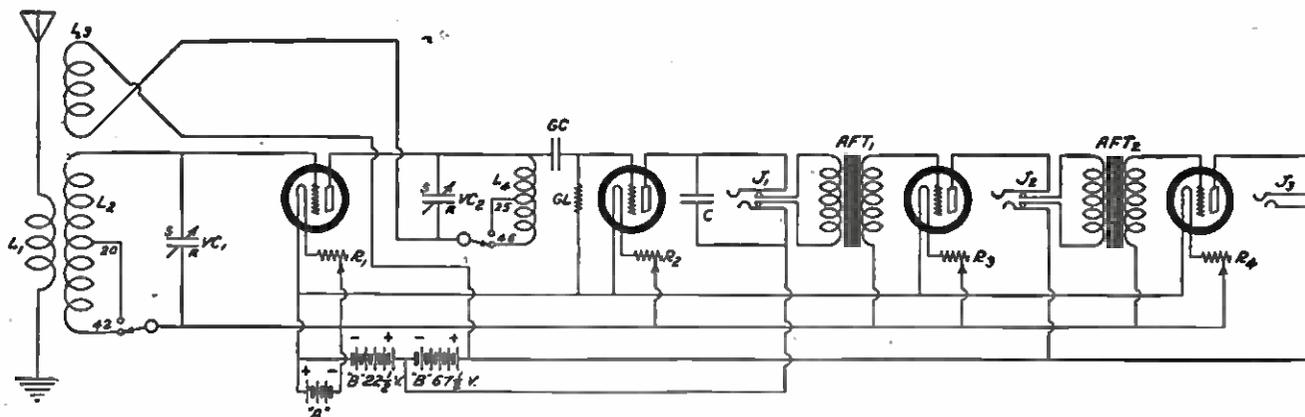
**THE SUPERDYNE CIRCUIT WHICH EMPLOYS A REVERSED-TICKLER FEED-BACK FOR ELIMINATING REGENERATION**
