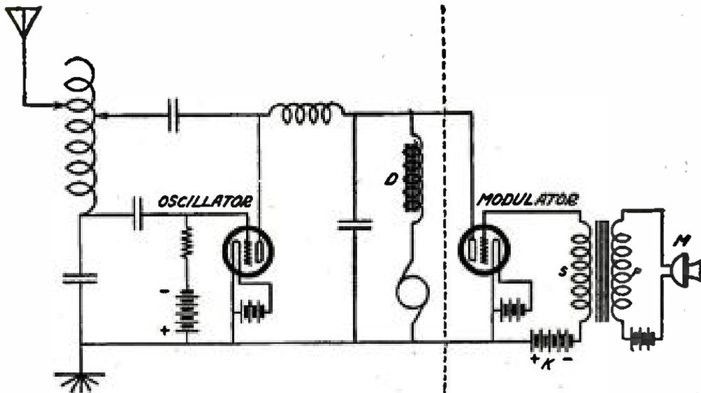
THE COLPITTS CIRCUIT WITH HEISING MODULATION
