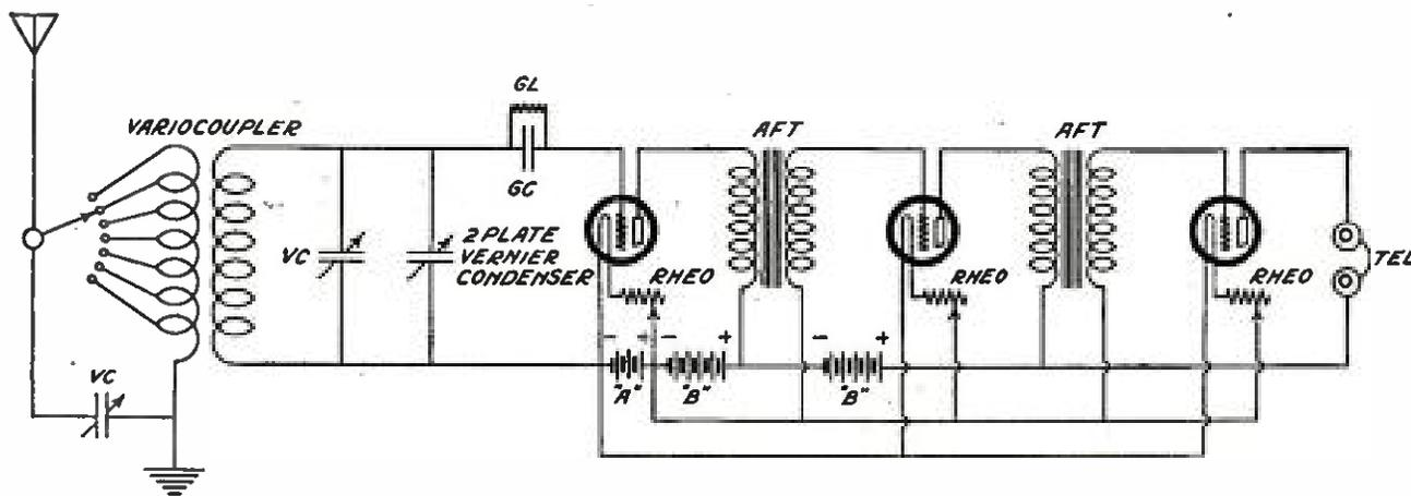
A SIMPLE AUDION CIRCUIT WITH TWO STAGES OF AUDIO-FREQUENCY AMPLIFICATION
