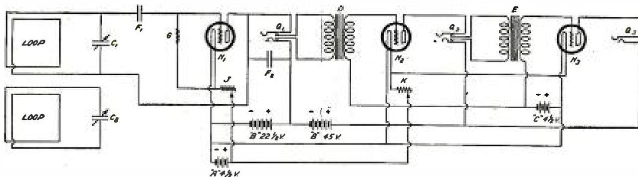
FOUR-CIRCUIT PORTABLE RECEIVER
