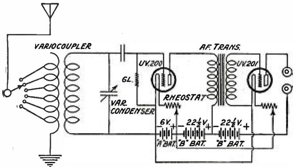
INDUCTIVELY-COUPLED, VACUUM-TUBE RECEIVER WITH ONE STAGE OF AUDIO-FREQUENCY AMPLIFICATION
