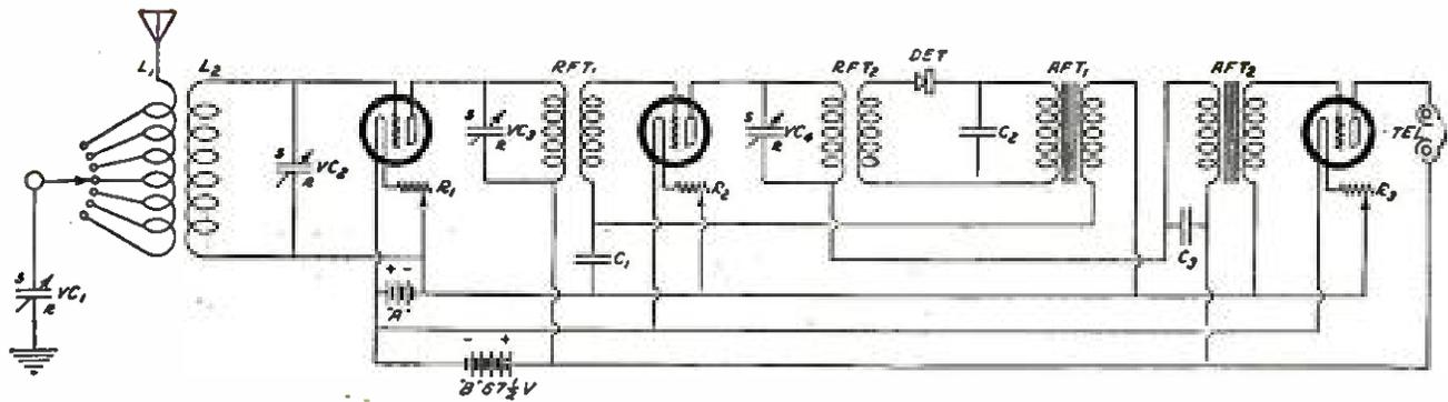
TWO STAGES OF TUNED-RADIO-FREQUENCY AMPLIFICATION, CRYSTAL DETECTOR AND TWO STAGES OF AUDIO-FREQUENCY AMPLIFICATION
