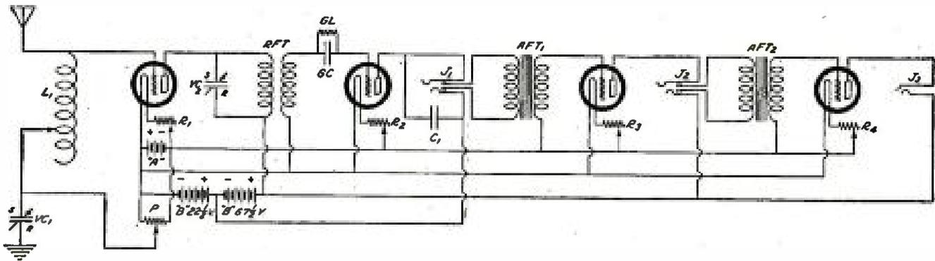
**SINGLE-STAGE RADIO-FREQUENCY AMPLIFIER WITH TUNED-PLATE CIRCUIT, DETECTOR, AND TWO-STAGE AUDIO-FREQUENCY AMPLIFIER**
