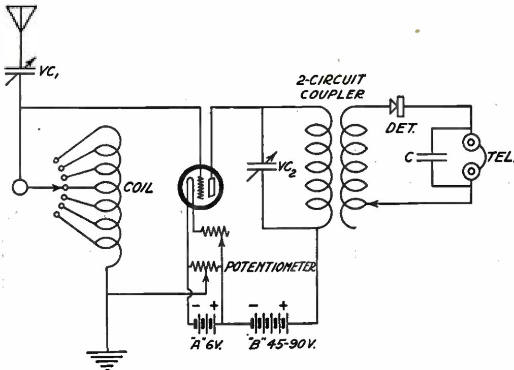
SINGLE-STAGE RADIO-FREQUENCY AMPLIFIER WITH CRYSTAL DETECTOR
