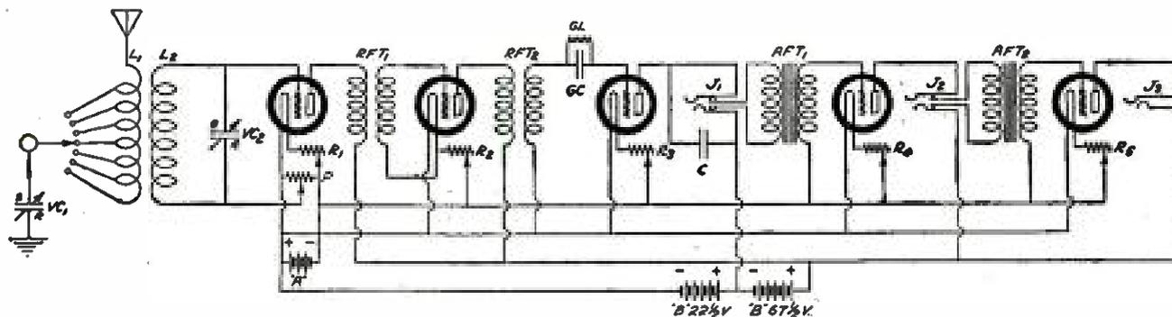
TWO STAGES OF TRANSFORMER-COUPLED RADIO-FREQUENCY AMPLIFICATION WITH VACUUM-TUBE DETECTOR AND TWO STAGES OF AUDIO-FREQUENCY AMPLIFICATION
