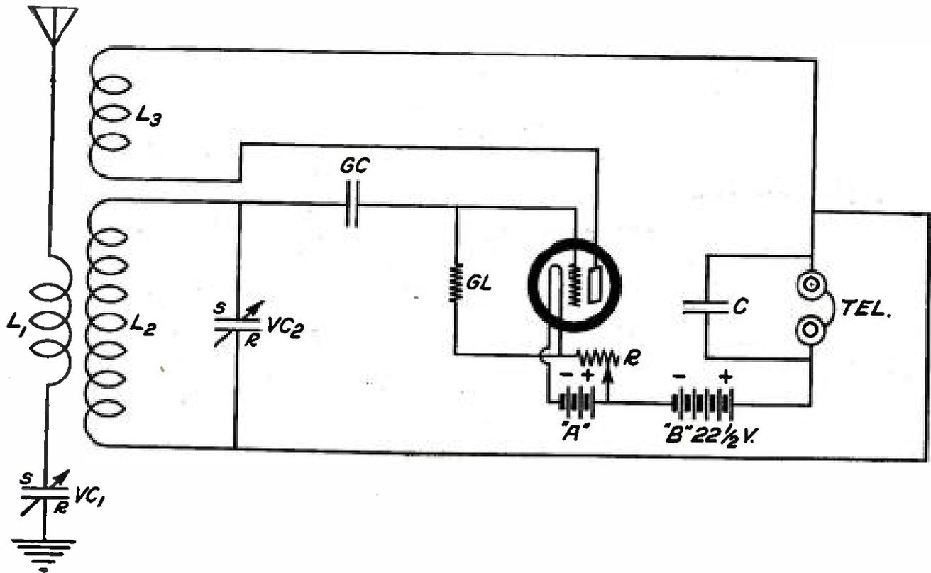
THREE-CIRCUIT TUNER FOR SHORT-WAVE RECEPTION
