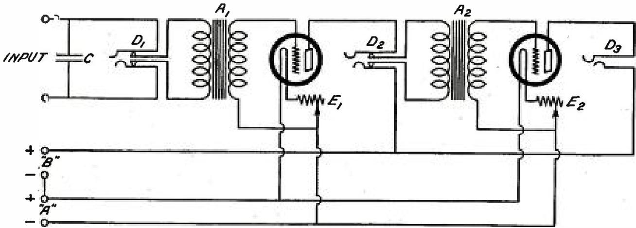
**TWO STAGES OF TRANSFORMER-COUPLED AMPLIFICATION**
