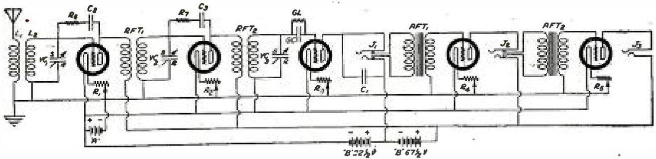
THE PLIODYNE PRINCIPLE INCORPORATED INTO A RADIO-FREQUENCY CIRCUIT WITH VACUUM-TUBE DETECTOR AND TWO-STAGE AUDIO-FREQUENCY AMPLIFIER
