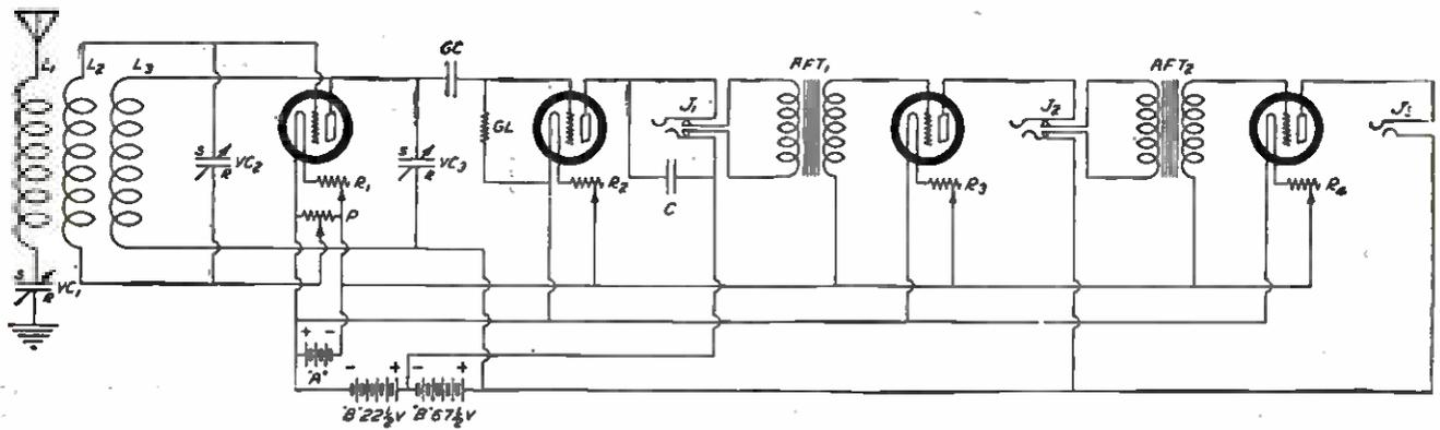
ONE STAGE OF TUNED-RADIO-FREQUENCY AMPLIFICATION, VACUUM TUBE DETECTOR AND TWO STAGES OF AUDIO-FREQUENCY AMPLIFICATION EMPLOYING HONEYCOMB COILS FOR TUNING
