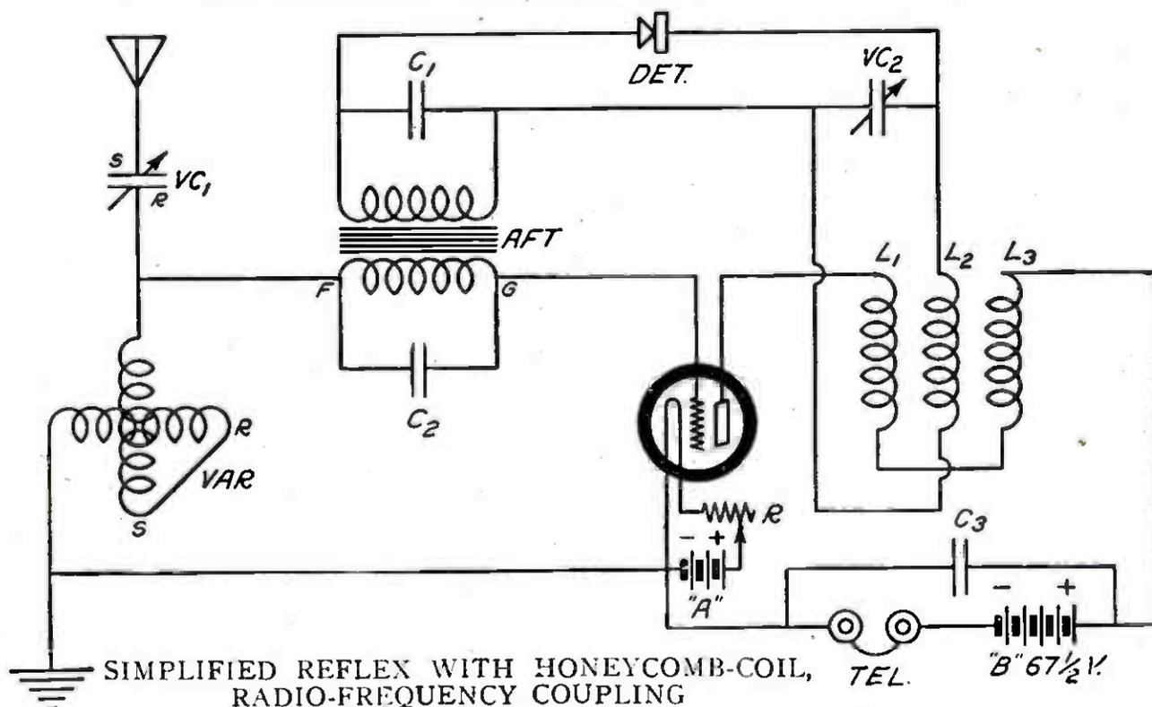
SIMPLIFIED REFLEX WITH HONEYCOMB-COIL, RADIO-FREQUENCY COUPLING
