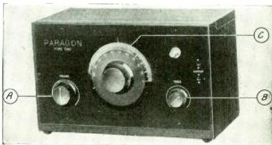
*A is the volume control. B is the detector rheostat. C is the tuning dial.*
