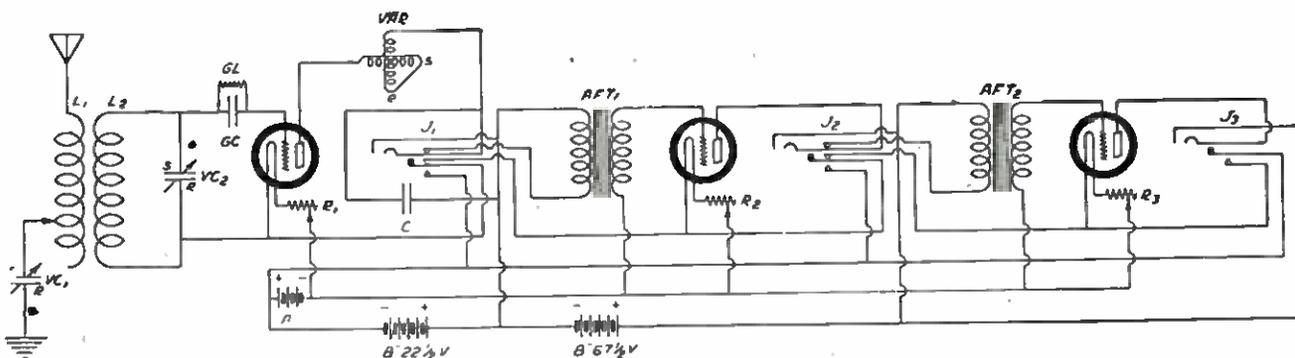
REGENERATIVE RECEIVER WITH TWO STAGES OF AUDIO-FREQUENCY AMPLIFICATION, EQUIPPED WITH AUTOMATIC FILAMENT-LIGHTING JACKS
