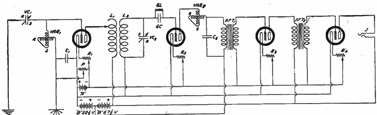
ONE STAGE OF TUNED-RADIO-FREQUENCY AMPLIFICATION, WITH A VACUUM-TUBE DETECTOR AND TWO STAGES OF AUDIO-FREQUENCY AMPLIFICATION
