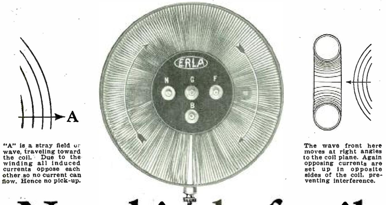
"A" is a stray field or wave, traveling toward the coil. Due to the winding all induced currents oppose each other so no current can flow. Hence no pick-up.
