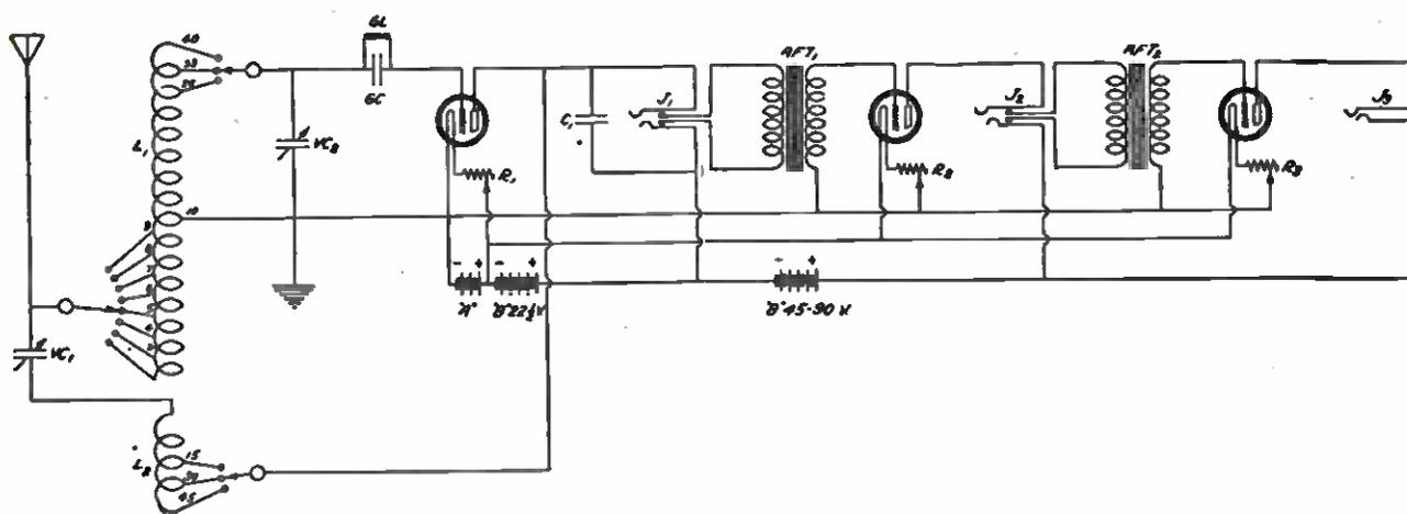
THE REINARTZ CIRCUIT, WITH TWO STAGES OF AUDIO AMPLIFICATION
