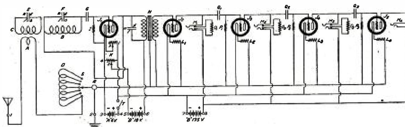
FOUR-CIRCUIT TUNER WITH ONE STAGE OF TRANSFORMER-COUPLED AND THREE STAGES OF RESISTANCE-COUPLED AMPLIFICATION
