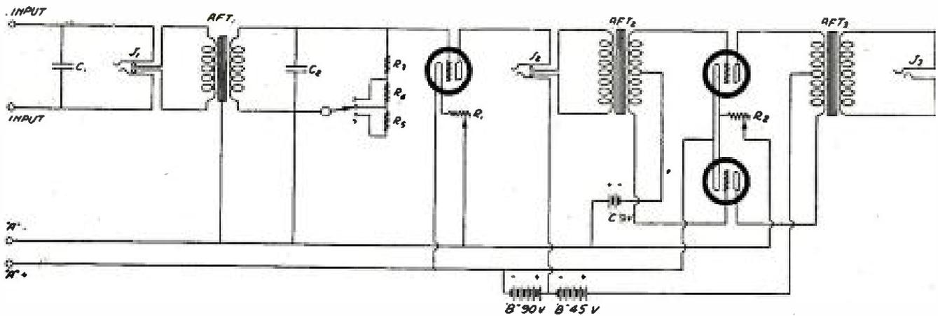
ONE STAGE OF TRANSFORMER-COUPLED, AND ONE STAGE OF PUSH-AND-PULL AMPLIFICATION
