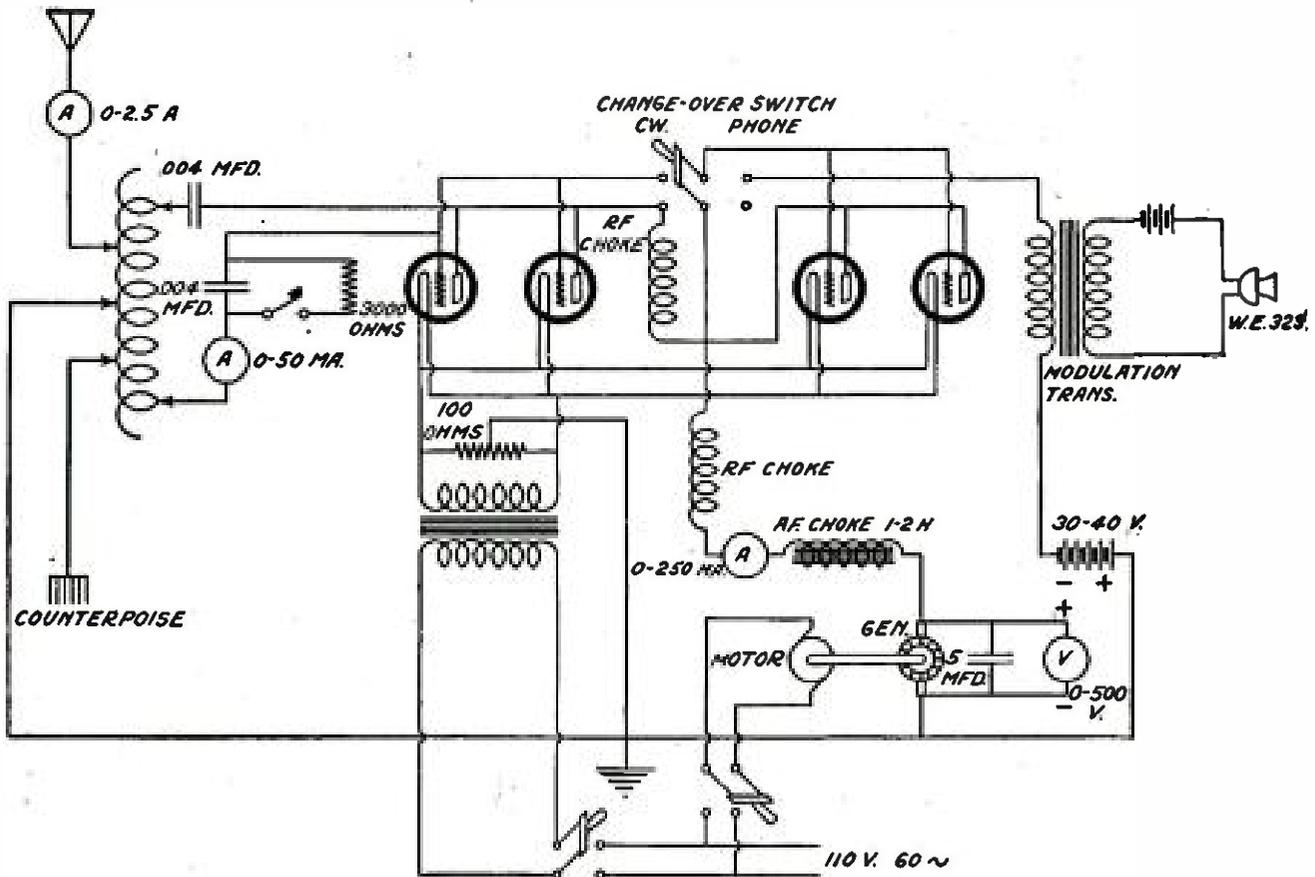
THE HARTLEY CIRCUIT USING HEISING MODULATION FOR TELEPHONY
