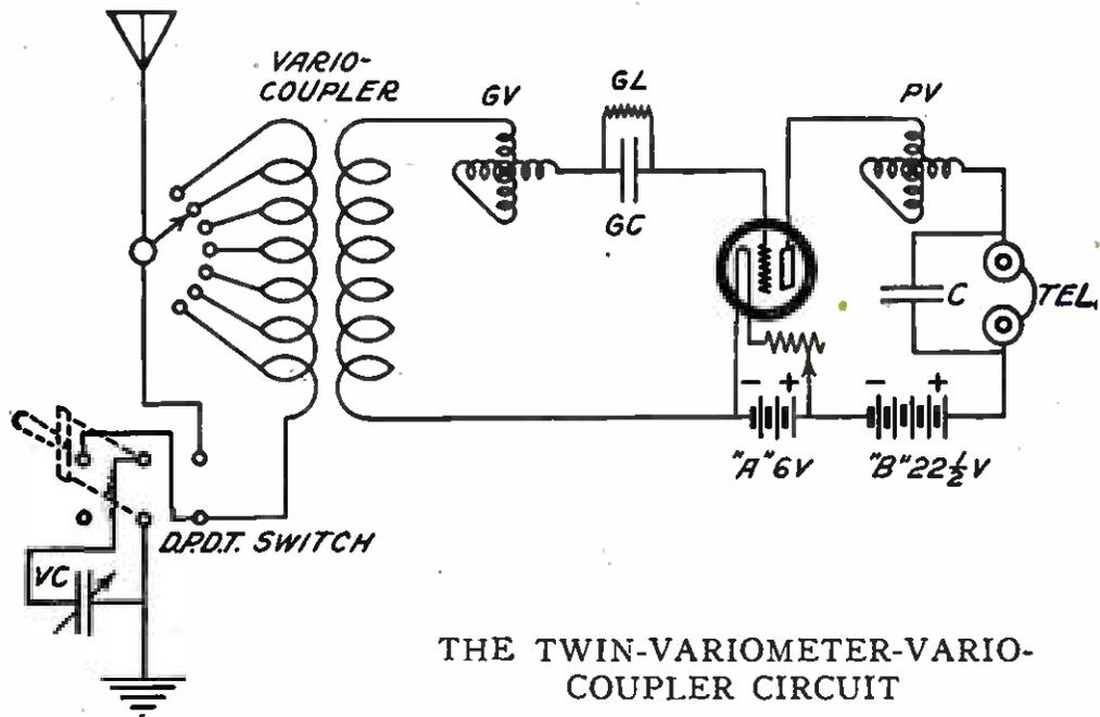
THE TWIN-VARIOMETER-VARIO-COUPLER CIRCUIT
