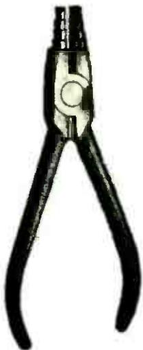
A complete and handy tool for electricians, radio set builders and mechanics. It will accurately form loops or eyes for No. 4, 6, 8 and 10 screws, make easy radius and sharp right angle bends, has flat jaws and wire cutters. This tool is made of the best quality steel, dropped forged and carefully tempered in oil.
