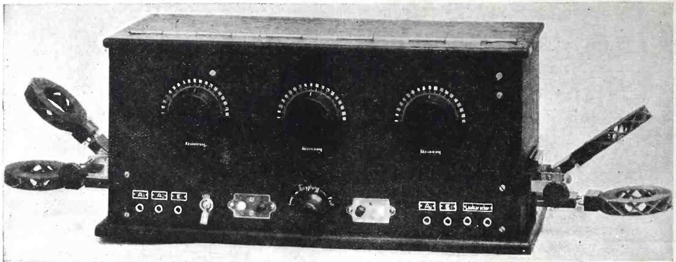
FIGURE 5: This is the set (the circuit of which is shown in Figure 4) which employs three valves that do the work of the average five-tube receiver.
