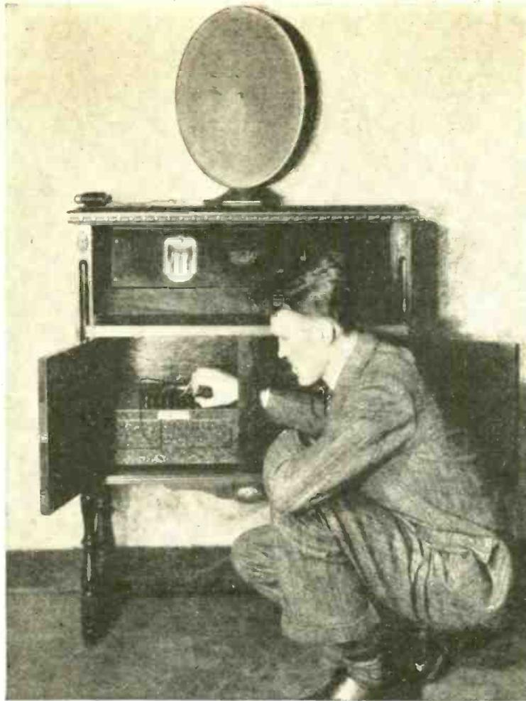
*The virtues of resistance coupling are fully realized when the LC-28 high-frequency pack is connected up with the National unit. The standard Corbett console cabinet of the LC-28 provides ample space for both the National unit and the "A" voltage supply.*
