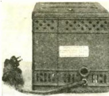
terminals to provide three "B" voltages, as required by most receivers, and the intermediate voltage is adjustable. The device will provide up to 196 volts at a current drain of 50 milliamperes.
