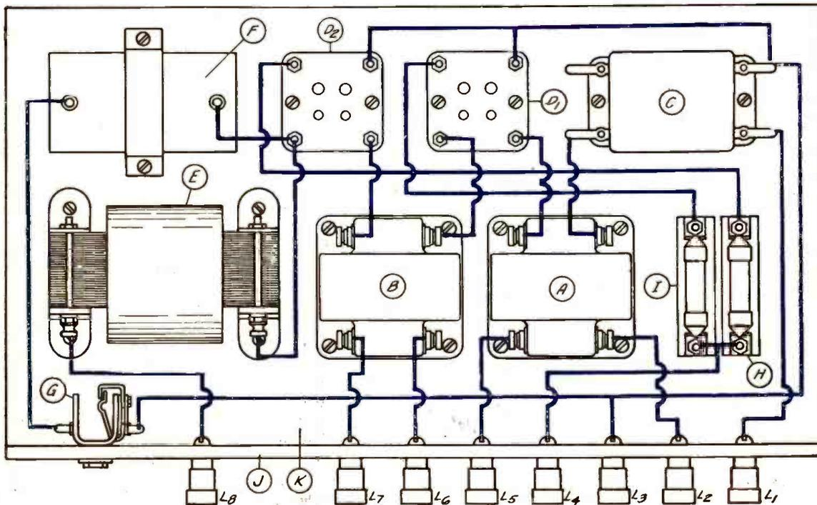
THE PICTURE WIRING DIAGRAM
