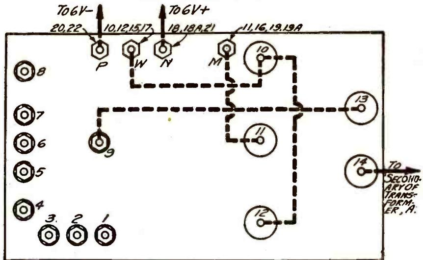
THE WIRING OF THE TOP PANEL
