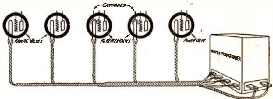
**THE FILAMENT WIRING FOR AC VALVES**
