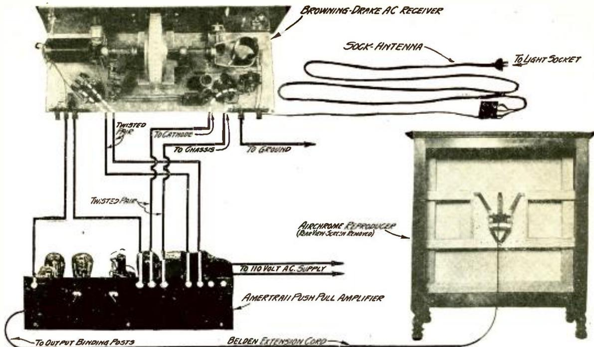
A COMPLETE SET-UP FOR THE AMPLIFIER
