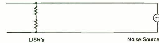
d) CM type I high frequency equivalent circuit
