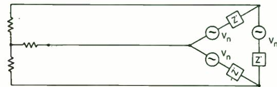
b) High frequency equivalent circuit for DM noise
