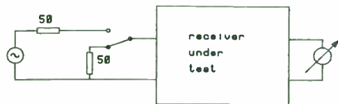
Fig. 12. Set-up for testing receiver performance.
