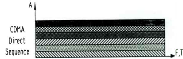
Figure 3. Code Division Multiple Access (CDMA)
