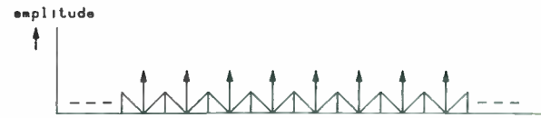
Fig.4. Uniformly crowded frequency spectrum of AM signals.
