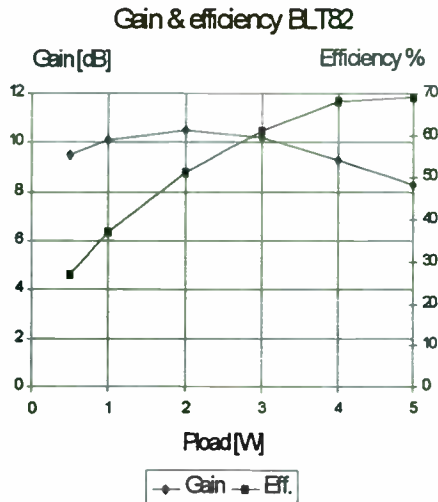
Fig.5 RF performance BLT82, 3.5 Watt transistor @ 6.0V, 900 MHz
