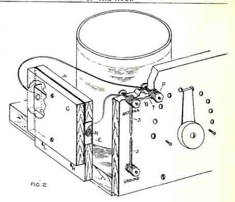
connected to this binding post. Another wire is connected to the terminal of the metal sheet C and led to the back of the binding-post P.
