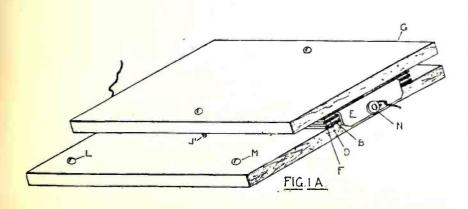
The wooden blocks are of dry wood smoothed up with sandpaper and given a coat or two of varnish which will not absorb moisture, or treated with paraffin as described in Cirular No. 120.
