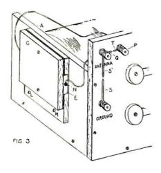
paper and thin metal are held carefully in position, and the cap block G is placed over them and screwed in position. The right end of the thin metal strip E is bent down, and a round head brass screw N is passed through a hole K, punched or drilled in the end of the metal strip. The projecting end of the strip C is not visible in Fig. 1A, but it is bent and fastened in the same manner as E. The completed condenser resembles the sketch shown in Fig. 1A.
