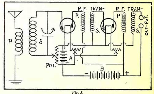
The potentiometer method of controlling the feedback is shown in the diagram above.
