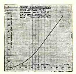
Fig. 3. A typical plate characteristic curve for the 199 type (3 volt) tube.
