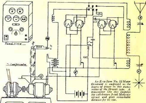
TO THE man who has a limited amount of capital to invest and wants to obtain the maximum miles per dollar, which is essentially the maximum miles per watt, this efficient little set should appeal. The set is a 20 watt transmitter using 4-5 watt tubes. By means of a double throw, double pole switch, the set may be used for either phone or continuous wave telegraphy. The circuit is the well-known three coil Meissner.
