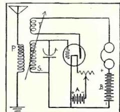
Fig. 1. Here current is induced in the secondary by a primary circuit. This secondary current acts upon the grid, which varies the current in the plate circuit. This varying current passes through the tickler coil which again causes an induced current in secondary, thereby affecting the grid once more, making a greater change in the plate circuit.
