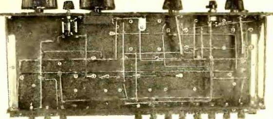
A bottom view of the super-heterodyne receiver, showing the wiring arrangement before the parts are installed. After studying this diagram and the others in this article, the fan should have no trouble in placing the parts. Every part is clearly marked by a number in the diagrams on the opposite page.
