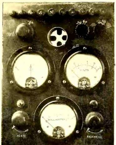
Fig 1. A front view of the vacuum tube tester, which can be made by any fan. Each part is so placed to give maximum efficiency, and no parts are used that will not be necessary. The tester is compact as well as attractive, and may be constructed for portable or stationary use.
