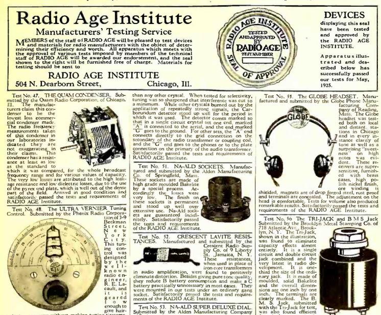
enough to give hair-give hair-ti is geared 20 to 1. The face of the dial remains from the vernier knob at the bottom of the dial. The real usefulness of this dial in quick and accu-rate tuning is the provision made for the fan to in-dicate on the dial with pencil or ink the station he desires. These units are very attractive in appear-ance. Satisfactorily passed the tests and require-ments of RADIO AGE Institute.
