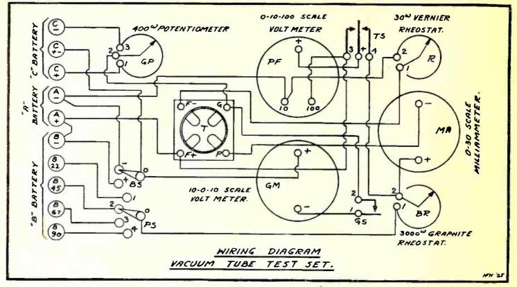
Fig. 2. Wiring diagram for Mr. Hopkins' tube tester. This layout is so simple a efficiency and worth are unlimited. Voltmeters of the highest rating were used in this unit. This layout is so simple any radio fan can follow it, and yet its
