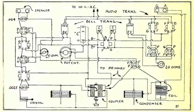
Complete wiring for a receiver operated on the A. C. house current. The only battery used is a 4 1-2 volt "C" battery—this being included in the set. There are five tubes in all; it's a three tube and crystal detector set, the extra two tubes furnishing the rectified current for the "B" voltage.
