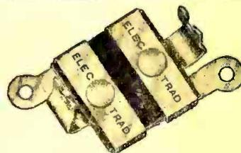
Test No. 83 submitted by the Electrad, Inc., 428 Broadway, New York. Sample consists of a grid condenser type G-S equipped with punched connecting lugs by means of which the condenser may be mounted directly to the socket. There are two prongs for the use of a cartridge resistance of a grid leak. The capacity of each condenser is stamped on the prongs. Tested and approved by the RADIO AGE Institute.
