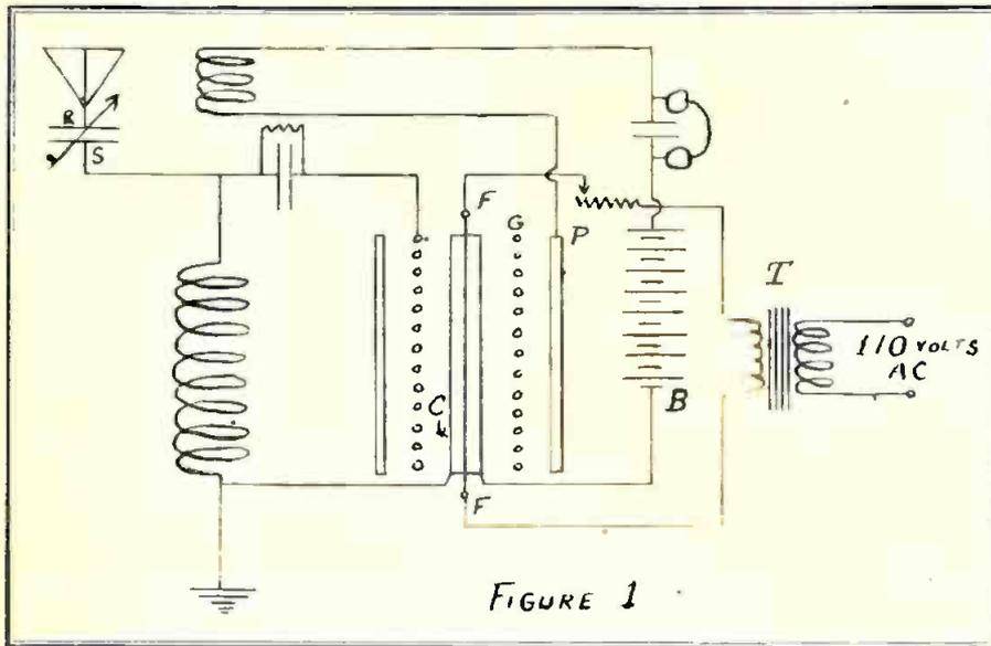
Fig. 1. Here is the schematic drawing for a typical alternating current tube supplied from the conventional 110 volt house supply. The filament F. F. is heated by the transformer voltage and in turn it passes its heat to the cylinder C which gives off an electronic emission.
