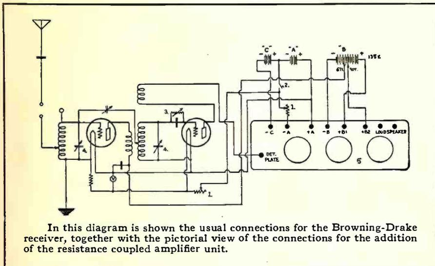
In this diagram is shown the usual connections for the Browning-Drake receiver, together with the pictorial view of the connections for the addition of the resistance coupled amplifier unit.
