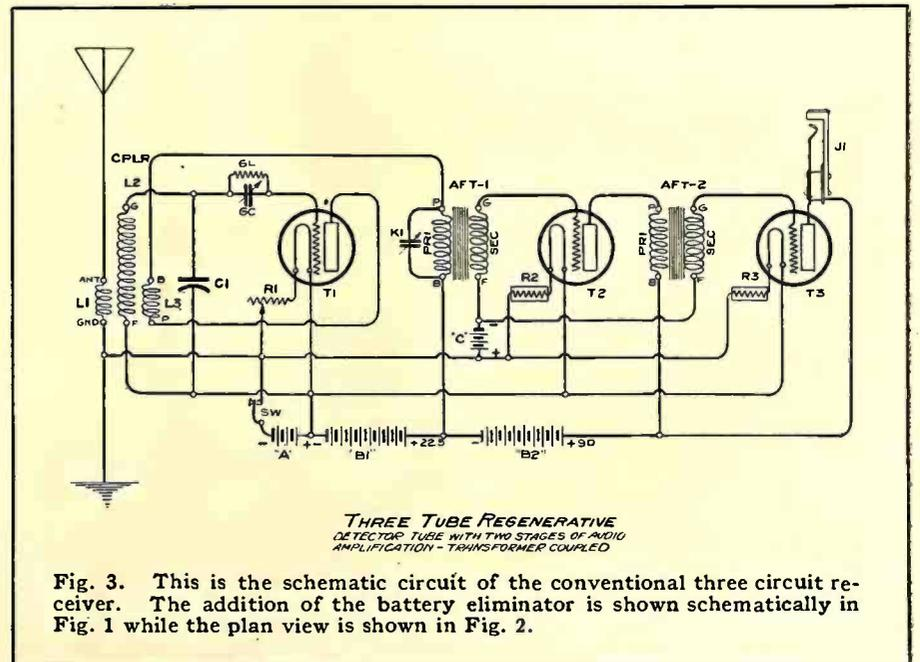
Fig. 3. This is the schematic circuit of the conventional three circuit receiver. The addition of the battery eliminator is shown schematically in Fig. 1 while the plan view is shown in Fig. 2.
