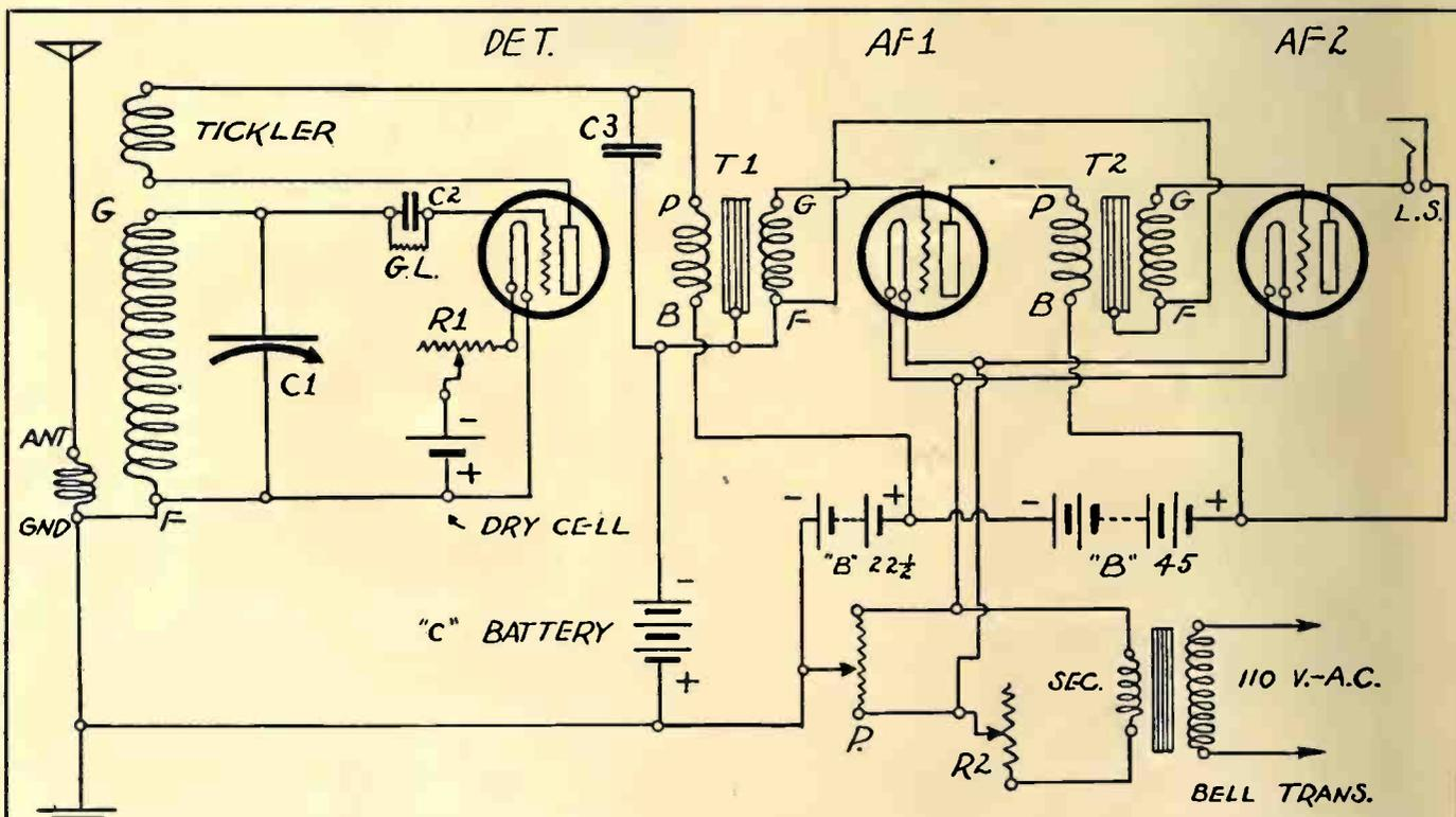
Fig. 1. Circuit diagram of a 3-tube receiver. The detector is a dry cell tube and the amplifiers are storage battery tubes lighted on alternating current through a transformer. The upkeep is greatly reduced in this way, without sacrificing results in the least.
