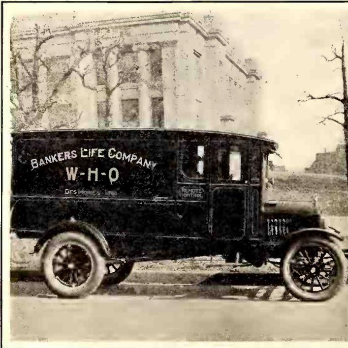
Remote control broadcasting is handled at WHO by means of an operator and the truck shown in the picture above
