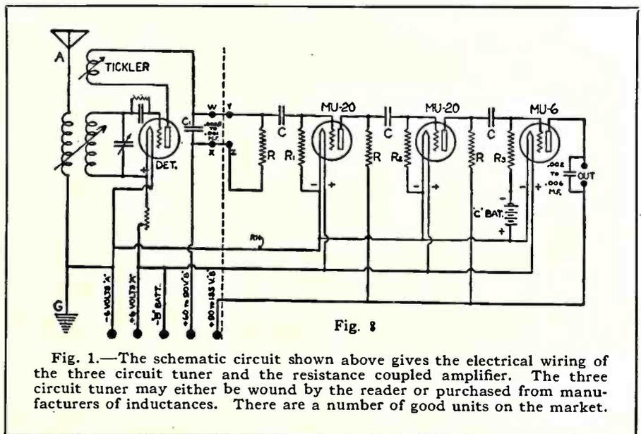
Fig. 1.—The schematic circuit shown above gives the electrical wiring of the three circuit tuner and the resistance coupled amplifier. The three circuit tuner may either be wound by the reader or purchased from manufacturers of inductances. There are a number of good units on the market.
