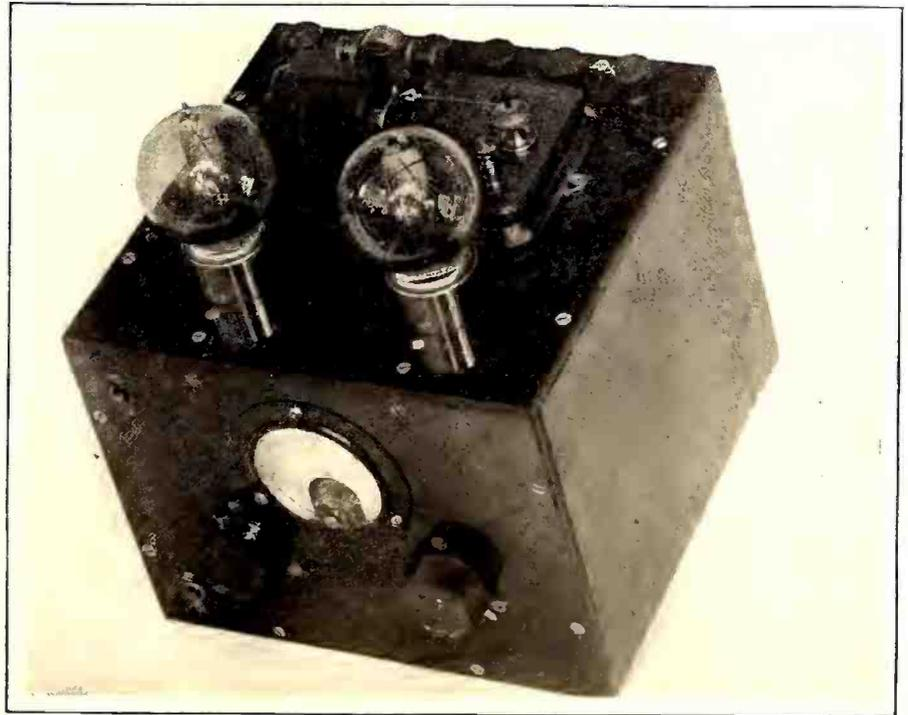
Amplifier and relay used on shipboard in radio-sound ranging. It is a two stage low frequency, transformer coupled set.
