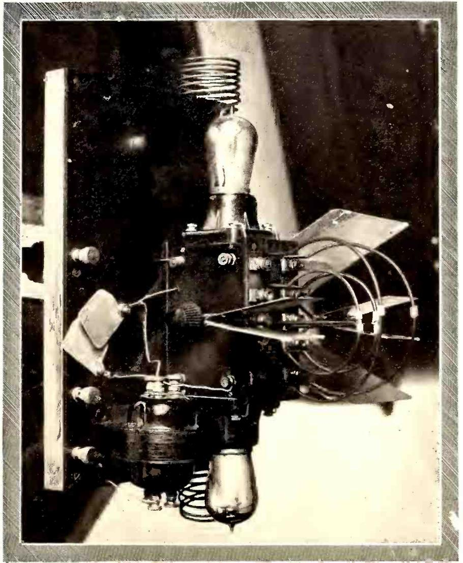
The complete radio transmitter which serves as the eye of the airplane is shown above. The wavelength used is 5 meters; the top helix being the antenna and the bottom one the counterpoise. The device is called the altimeter and accurately gauges the deviation of aircraft from a predetermined height
