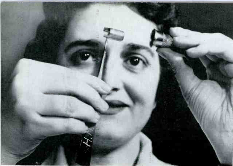
Rugged "Nuvistor" tube is small enough to fit in thimble.
