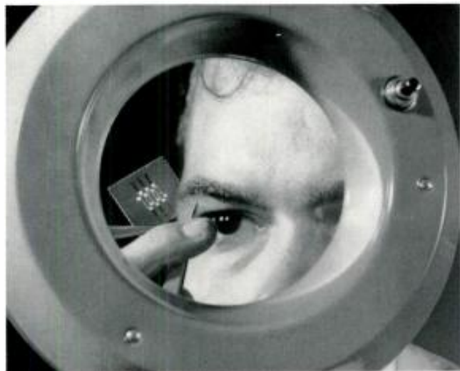
Thin-film transistor promises computer circuits of book-page size.
