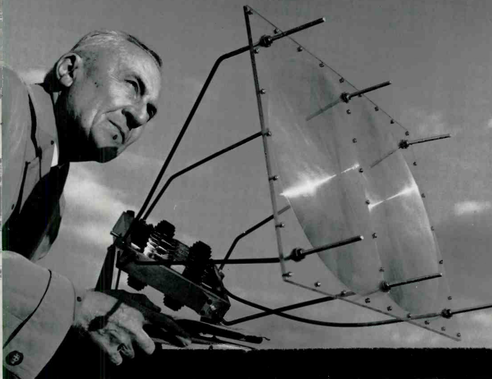
RCA's N. E. Lindenblad tests behavior of thermoelectric materials by focusing solar heat through special lens on a small test motor.
