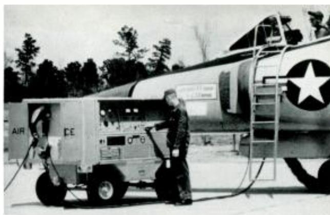
*RCA's DATS system checks out aircraft fire-control.*
