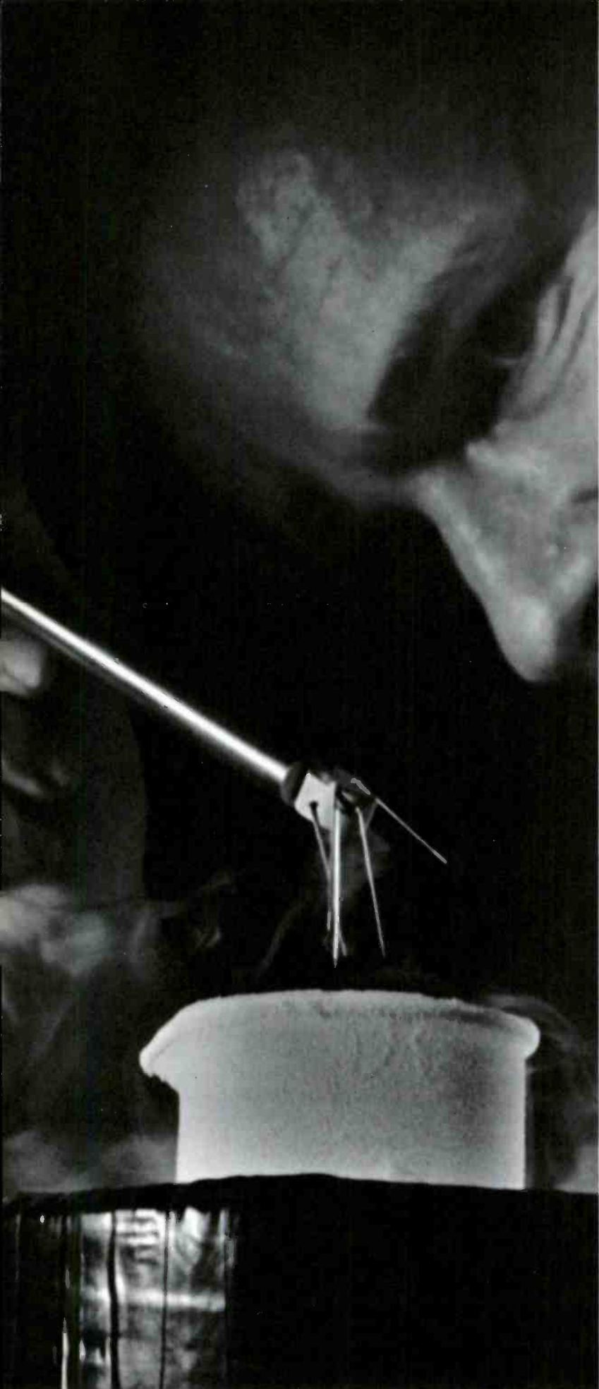
Pins adhere to this cadmium-chromium selenide slug, which becomes a powerful ferromagnet when cooled to minus 321 degrees F.
