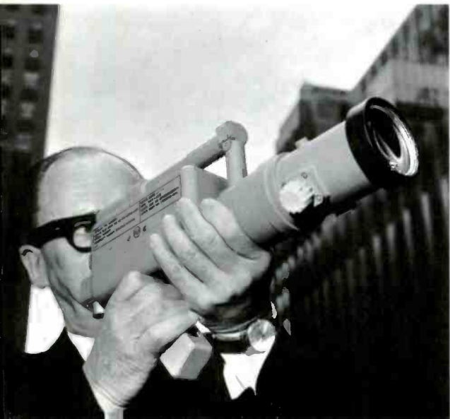
Above left, RCA's new dielectric tape camera system that has been developed for use in mapping distant planets, weather surveillance, and other space missions.
