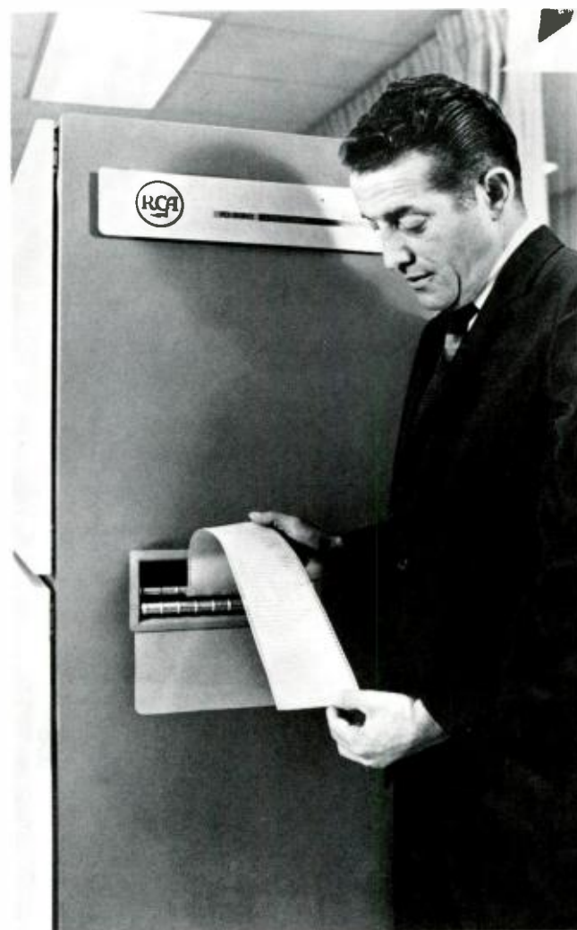
RCA's Videocomp system produces printed material at the rate of 650 characters a second.
