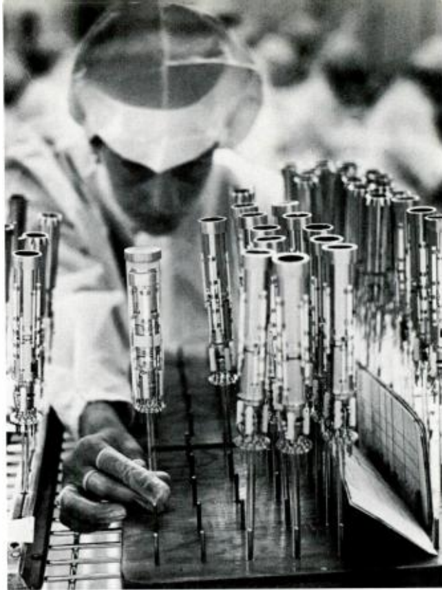
A group of supersensitive RCA television camera tubes used in the Navy's air-to-surface "Walleye" weapon near completion.
