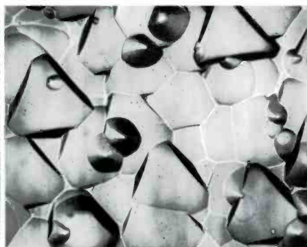
Various microscopic views of single crystals whose surfaces have been etched to reveal defects and structural details of importance to their electronic properties.
