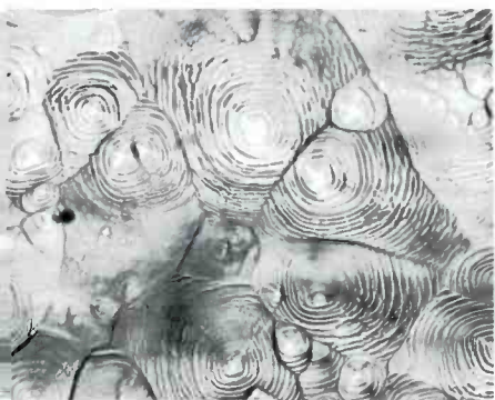
Various microscopic views of single crystals whose surfaces have been etched to reveal defects and structural details of importance to their electronic properties.
