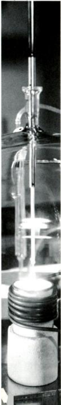
A single crystal of calcium tungstate being drawn from a melt.
