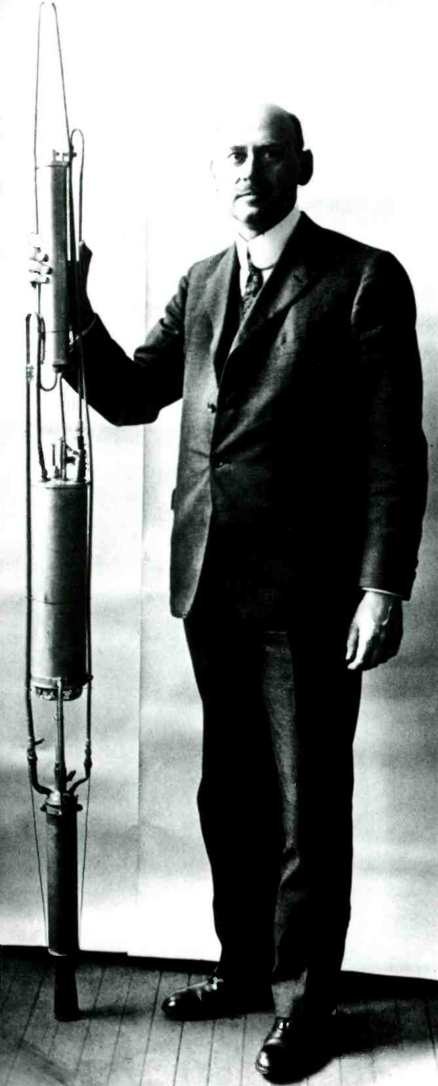
Goddard with his liquid-fueled rocket: the motor is at the base and the fuel tanks are above it.
