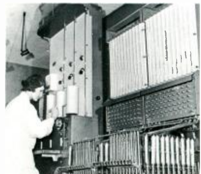
Russian technician checks a hydraulic integrator, a computing device for the construction industry.
