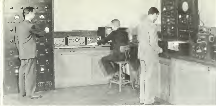
LEFT: DR. H. F. OLSON ARRANGES APPARATUS FOR ACCURATE TESTS OF AN ARTIFICIAL VOICE IN RCA LABORATORIES' FREE-FIELD SOUND ROOM. RIGHT: IN THIS ROOM ENGINEERS WATCH INSTRUMENTS WHICH RECORD THE QUALITY CHARACTERISTICS OF A LOUDSPEAKER UNDER TEST.
