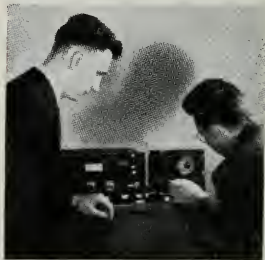
The RCA radio altimeter will be a major contribution to the safety of post-war commercial flying. The section at the left sends the radio waves to earth and back again while the "box" at the right—timing these waves to the millionth of a second—tells the navigator the plane's exact height in feet.
