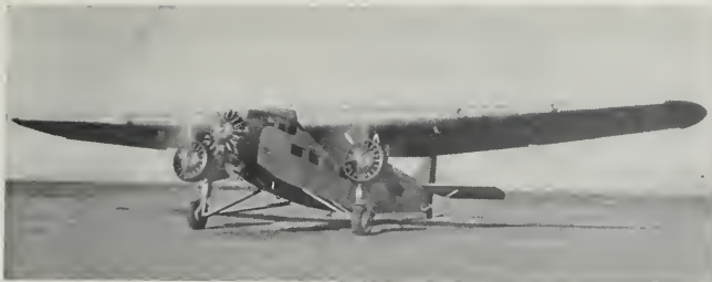
PLANE USED BY RCA FOR ITS OBSTACLE DETECTION TESTS IN 1937-39. THE V-ANTENNA APPEARS JUST ABOVE THE CENTER OF THE WING-SPAN.
