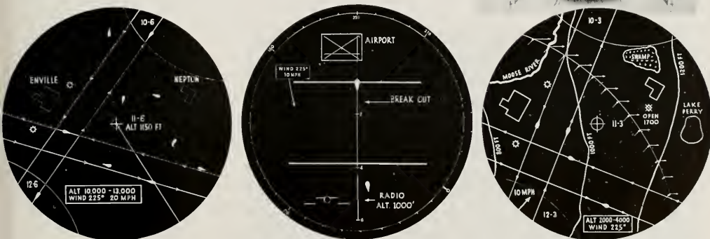
BELOW, LEFT TO RIGHT: FIGURE 2—TYPICAL PICTURE SENT ALOFT BY TELERAN; FIGURE 3—PICTORIAL INSTRUCTIONS WHICH GUIDE PILOT IN LANDING; FIGURE 4—TELERAN WEATHER MAP AND TERRAIN FEATURES. AT RIGHT: FIGURE 5—SUGGESTED METHOD OF MOUNTING TELERAN KINESCOPE IN COCKPIT OF PLANE.
