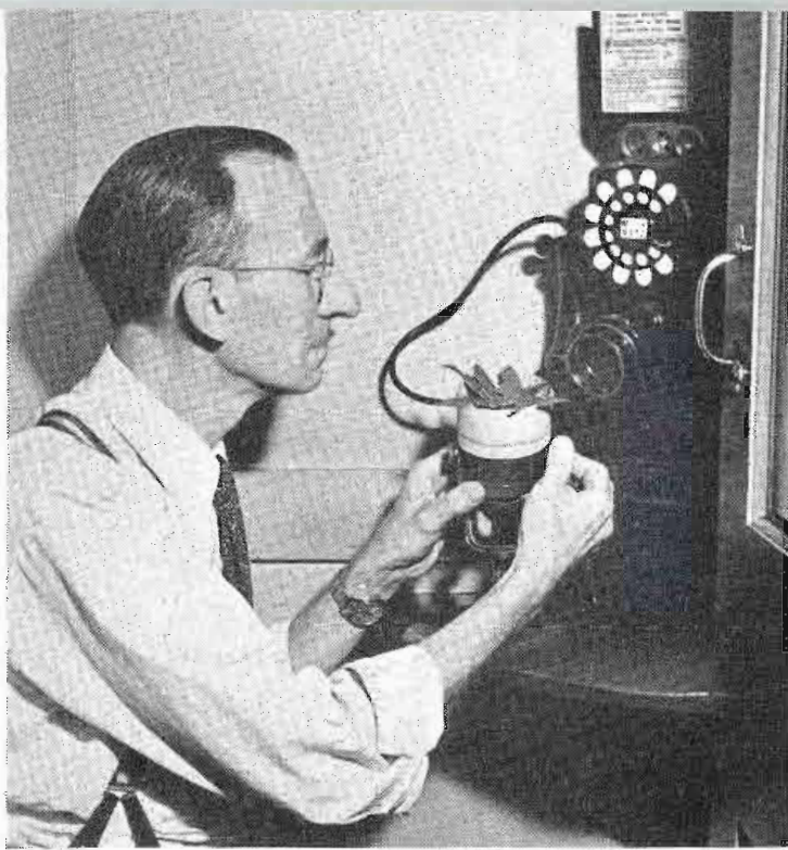
A telephone booth provides the minimum atmospheric noise for recording the delicate sounds of beetles chewing leaves.
