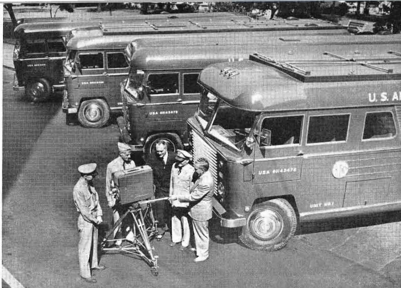
Four huge vans comprise the modern "TV station on wheels" developed by RCA for the U. S. Army Signal Corps.
