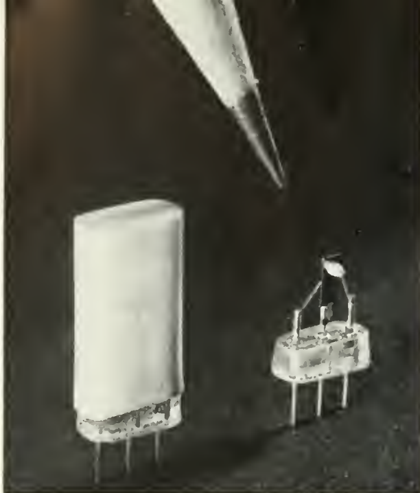
Developmental junction-type transistor before and after embedment in plastic container, shown here in comparison with pencil point.
