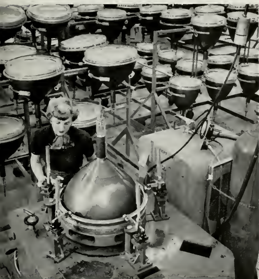
Welding a 19-inch tricolor tube at the Lancaster, Pa., RCA plant, where tube is in pilot production.
