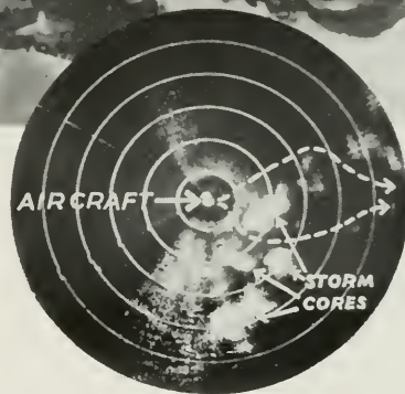
In the drawing above, a United Air Lines plane peers through a storm with RCA's airborne weather radar unit. Photo of radar screen at right shows how the pilot can find route that avoids storm cores.
