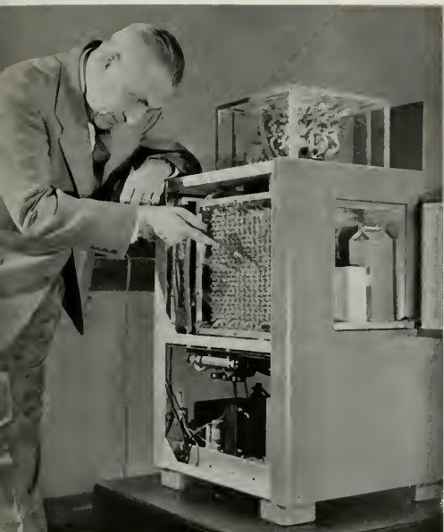
Nils E. Lindenblad, who directed development of RCA's electronic cooling system at the David Sarnoff Research Center, points out a feature of the experimental electronic refrigerator.
