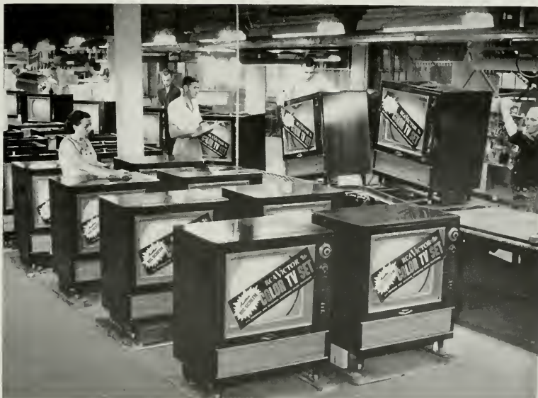
On the production line at Bloomington, Ind., RCA Victor 21-inch color TV sets are readied for shipment after final tests.
