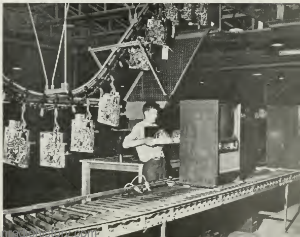
Chassis and cabinet meet on the television assembly line at the Prescott, Ontario, plant.
