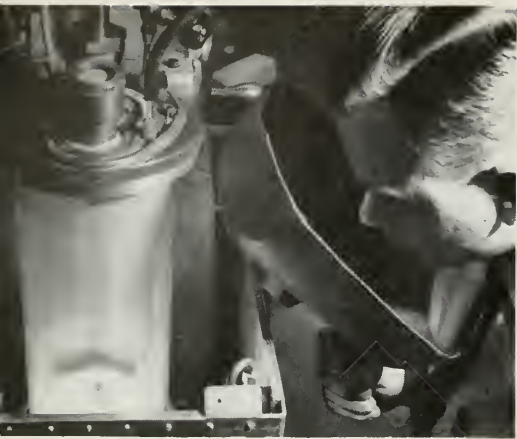
An operator observes the formation of a developmental silicon crystal in the Materials Laboratory.
