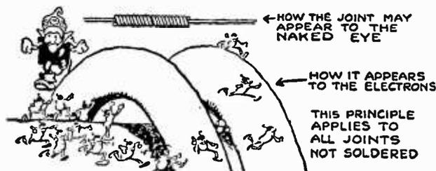
King Electron can quickly determine the condition of the various parts.
