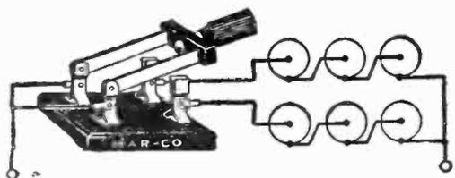
**E**CONOMICAL operation of UV 199 tubes requires a series-multiple connection of dry cells. Difference in age and voltage existing between separate series lines will cause current to flow through the multiple connections even when the battery is apparently standing idle, ruining the cells and causing them to disrupt and discharge electrolyte to cause damage.
