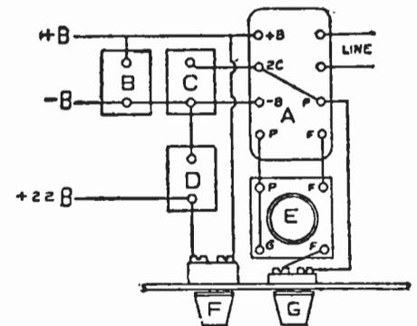
Method of wiring Type B. T. 200 Transformer for "B" Battery supply using 110v-60 cycle AC Line.
