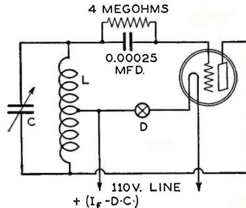
Fig. 3—A simple oscillator for general testing purposes.
