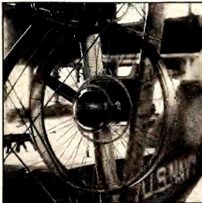
View of a wind-driven motor generator.
