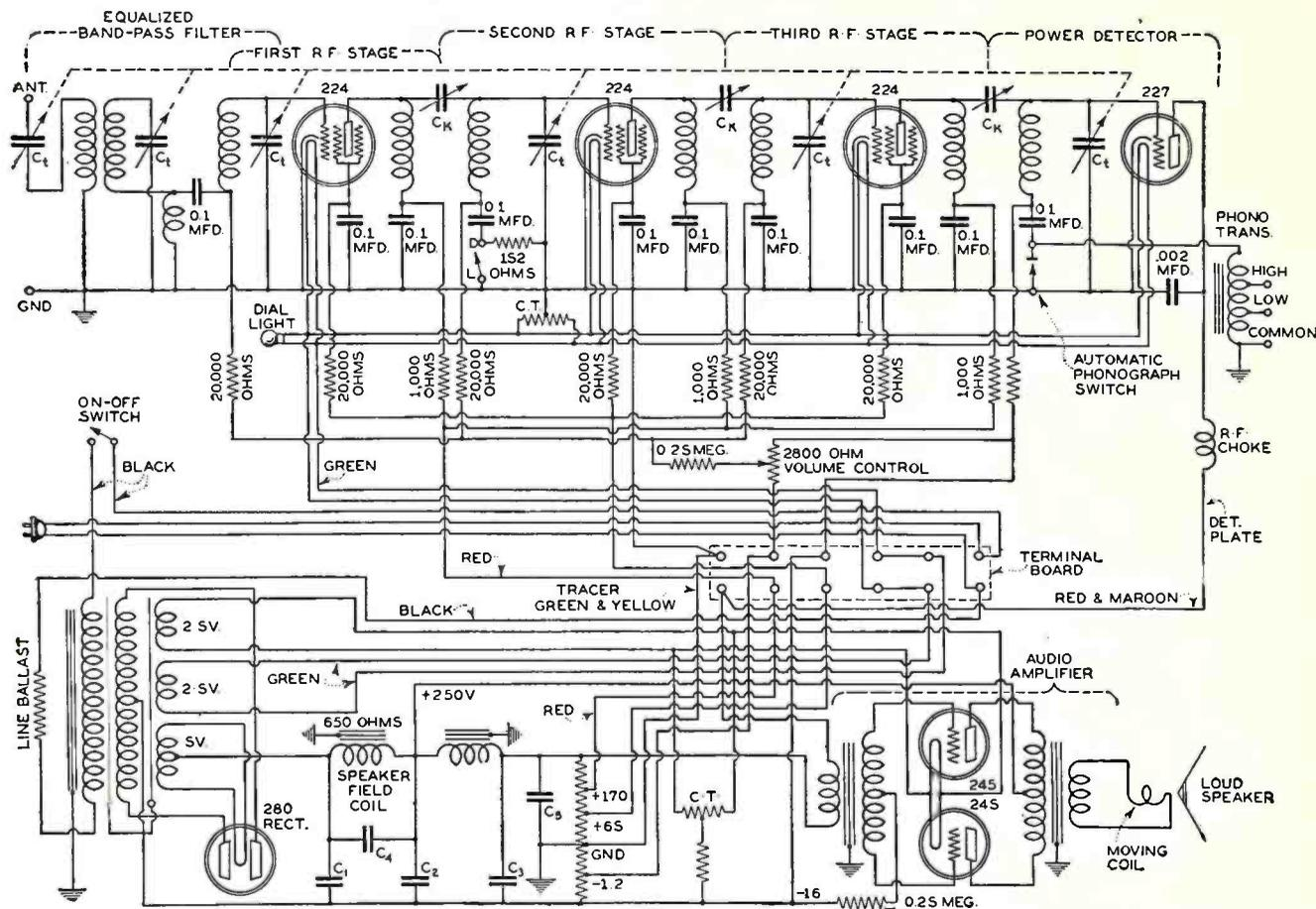
THIS RECEIVER consists of a three-stage screen-grid r.f. amplifier, a type 227 detector, and a push-pull output stage using two 245-type tubes supplying power to an electrodynamic loud speaker. The receiver contains several unusual features.
