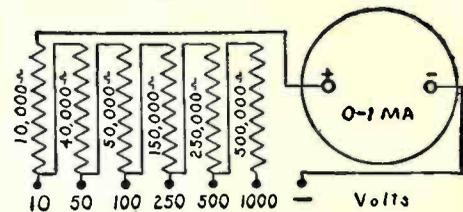
The Super Akra-Ohm wire-wound Resistor is especially adapted for use as a Voltage Multiplier as shown in the above diagram. It is carefully designed to insure an accuracy of 1 per cent and a constant permanency of calibration. Its use is also highly recommended for Laboratory Standards, High Voltage Regulators, Telephone Equipment, and Television Amplifiers, Grid and Plate Resistors, etc.
