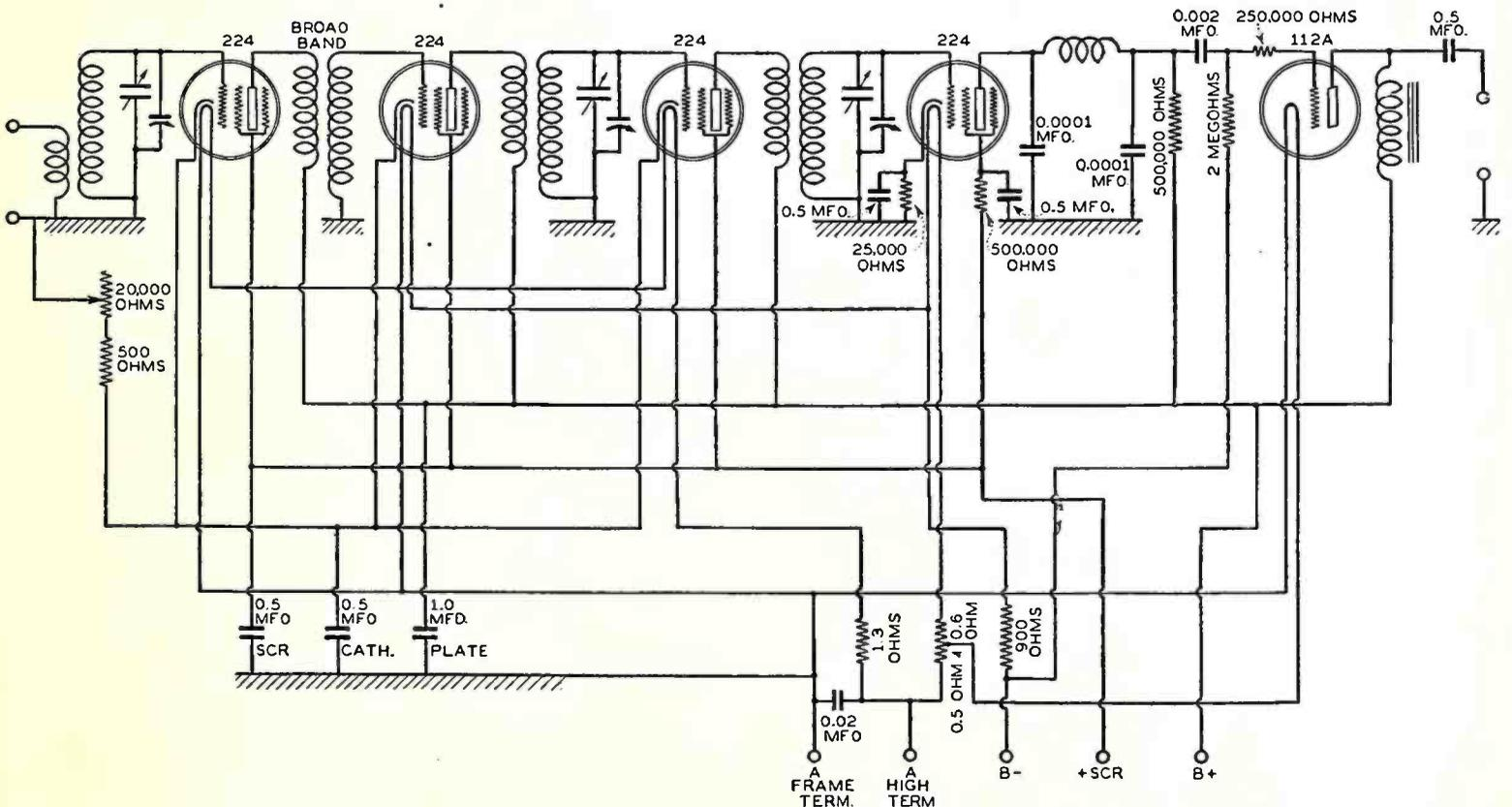
Fig. 3—The complete schematic diagram of the Bosch motor car receiver chassis.
