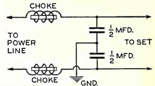
Fig. 2—Using r.f. chokes for additional filter action.
