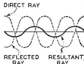
The curves on this sheet indicate graphically the effects which occur due to the direct and reflected rays. If the two waves are essentially 180 degrees out of phase the resultant, shown by the heavy line, is very small which means that the intensity of the sound is very low. However, reflection is not always a thing to be avoided. For example, it occurs in an auditorium and often adds atmosphere to the music being played.
