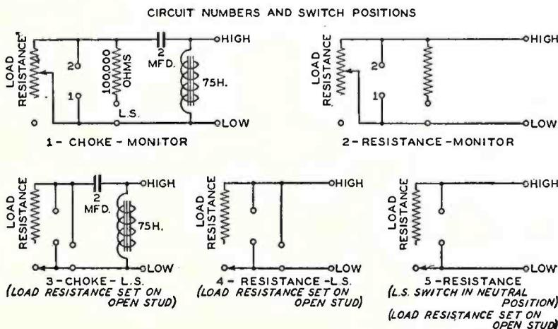
Fig. 2—Circuits obtainable with loading device.
