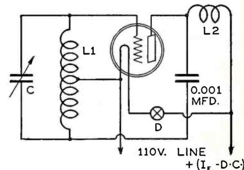
Fig. 4—A variation of Fig. 1 with parallel feed.
