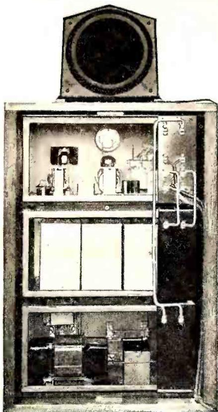
Rear view of audio-frequency voltmeter.
