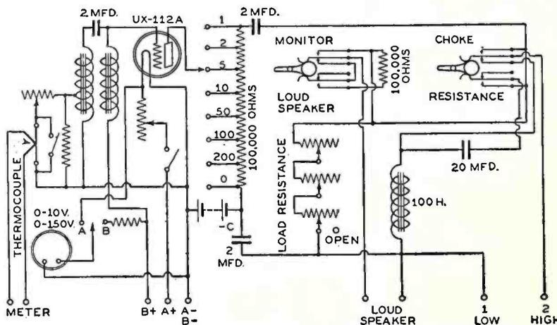
Fig. 1—Circuit of A.F. voltmeter and loading device.
