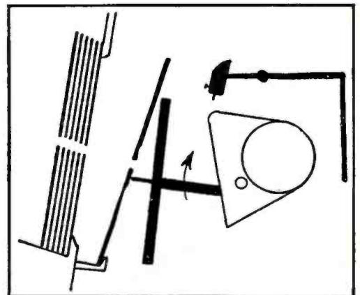
**Fig. 4—Step three: turntable rising to pick up record ejected from magazine.**
