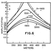
Due to the fact that the feedback originating in the fourth stage can feed back through three stages, and that originating in the third stage can feed back through two stages, and so on, it is clear that the regeneration conditions cannot be the same in all
