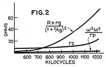
This is the amplification equation of the circuit of Fig.1C, which may, therefore, be regarded as the approximately equivalent circuit of the amplifier. The manner in which the three components of the equivalent resistance vary with frequency is shown in Fig. 2, which has been calculated for a typical case. Likewise, in Fig. 3, there is shown a curve of voltage amplification, calculated by equation (8)
