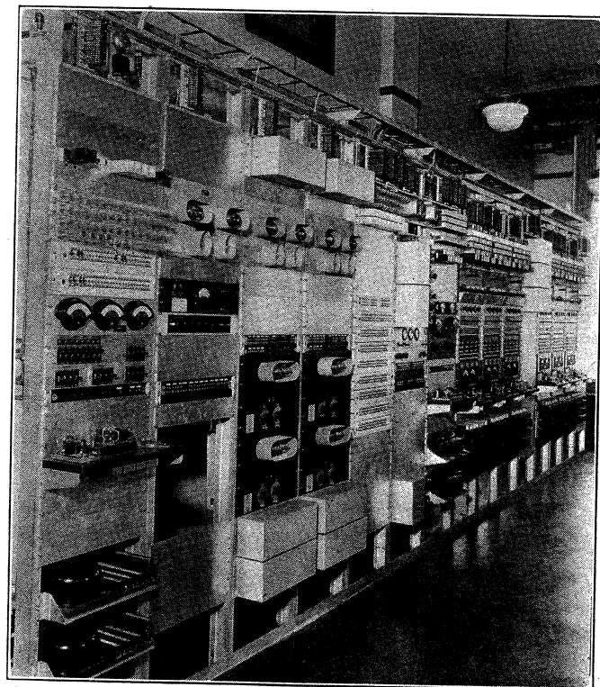
Fig. 8. Equipment for one terminal of 24-channel system.
