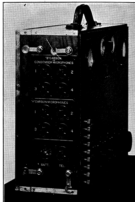
Fig. 3. End view of 30-A portable amplifier showing the two groups of microphone receptacles.
