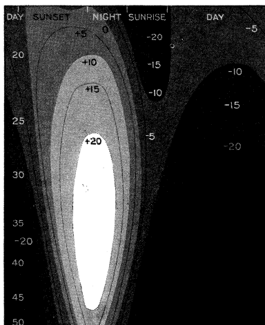
Fig. 1. Average field strength surface for June, 1926, db. above 1 microvolt per meter for 1 kw. radiated.
