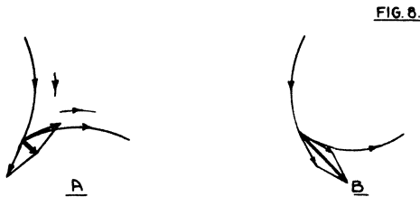
Fig. 8A shows how the components of two pincushion fields add together and give a comparatively small resultant for corner deflection and a barrel shape pattern. Similarly the components of two barrel shape fields add together as shown on Fig. 8B and give a comparatively large resultant and a pincushion pattern.
