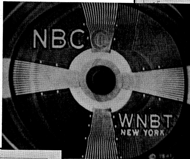
FIG. 10, BELOW. IN THIS CASE THE REFLECTION IS FROM AN OBJECT NEAR THE TRANSMITTER. THIS ALSO CAUSES A FIXED GHOST AT THE RECEIVER. FIG. 12A, RIGHT. ACTUAL PHOTO OF A FIXED GHOST, DISPLACED TO RIGHT OF MAIN PATTERN
