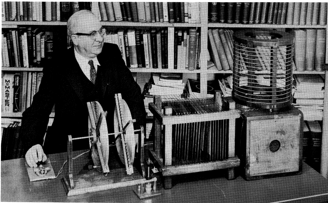
The fifty-year old spark gap of this wireless transmitter, pounds out the introductory message of the Golden Jubilee LP Record. Harry Houck, owner and builder of the equipment, is the operator.
